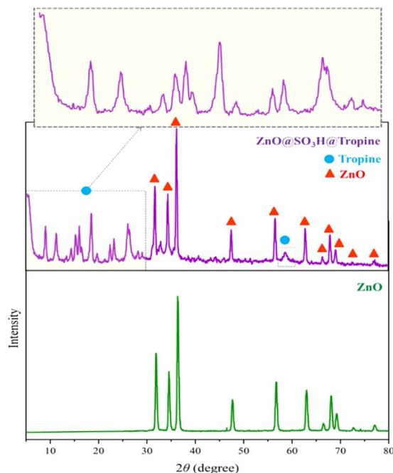
Fig. 4 XRD patterns of ZnO and ZnO@SO<sub>3</sub>H@Tropine.
