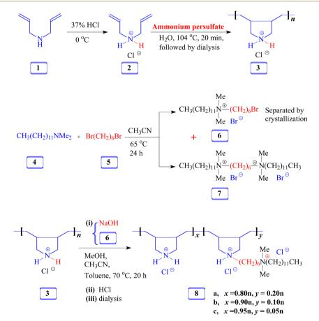
Scheme 1 Synthesis of the diallylamine salt-based monomer cyclopolymers.
