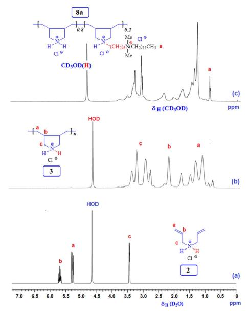
Fig. 2  $^{1}$ H NMR spectra of (a) 2 in  $D_2O_2$ , (b) 3 in  $D_2O_2$ , and (c) 8a in  $CD_3OD_2$
