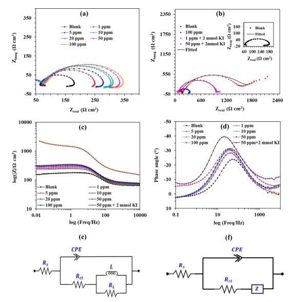
Fig. 8 (a) Nyquist plots for mild steel corrosion in 20% formic acid in the presence and absence of different concentrations of 8b; (b) Nyquist, (c) Bode magnitude, and (d) phase angle plots for 8b in the presence and absence of 2 mmol KI; equivalent circuits used to fit Nyquist plots associated with the usage of 8b (e) without and (f) with KI.
