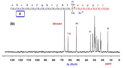
Fig. 1 (a) <sup>1</sup>H and (b) <sup>13</sup>C NMR spectra of salt 6 in D<sub>2</sub>O.
