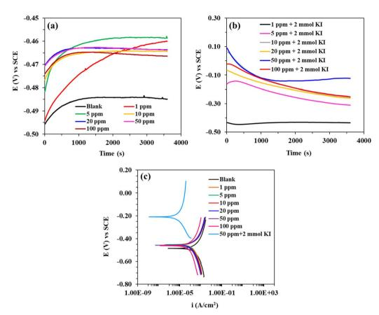
Fig. 7 OCP vs. time curves for mild steel corrosion in 20% formic acid containing **8b** in the (a) absence, (b) presence of 2 mmol KI, and (c) Tafel plots in the presence and absence of different concentrations of **8b** with and without 2 mmol KI.
