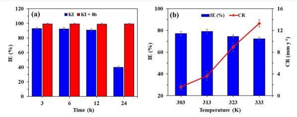
Fig. 6 (a) Variation of the IE of KI and **8b** (50 pppm) with 2 mmol KI at different time intervals at 60 °C; (b) impact of temperature (303–333 K) on the IE imparted by **8b** (100 ppm).
