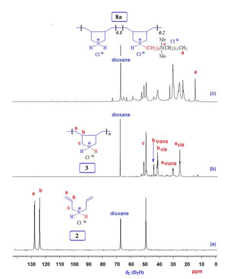
Fig. 3  $^{13}$ C NMR spectra of (a) 2 in D<sub>2</sub>O, (b) 3 in D<sub>2</sub>O, and (c) 8a in CD<sub>3</sub>OD
