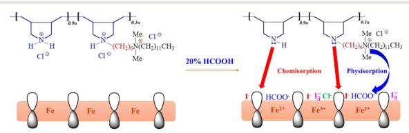
Fig. 12 An illustration of PDAAC undergoing adsorption on the mild steel surface.
