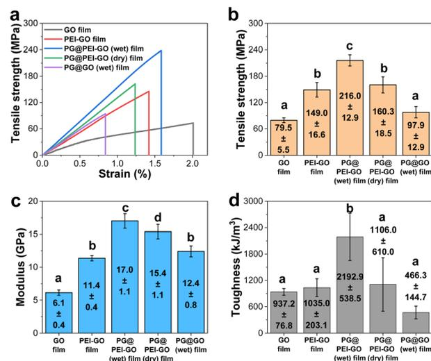
Fig. 4 (a) Stress–strain curves, (b) tensile strength, (c) modulus, and (d) toughness of GO, PEI-GO, PG@PEI-GO (wet), PG@PEI-GO (dry), and PG@GO (wet) films. Error bars represent the standard deviation (at least  $n = 3$ ); different letters represent significantly different means ( $p < 0.05$ ).
