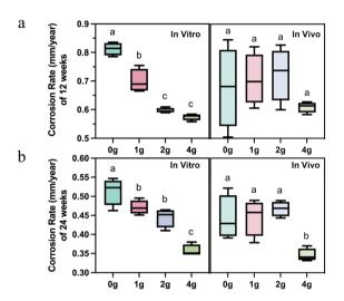
Fig. 3 The *in vitro* and *in vivo* corrosion rate of the HP magnesium rods with different designs at 12 (a) and 24 weeks (b) post-operation (n = 4). Columns significantly different letter (p < 0.05) to each other would be labeled with different letters.
