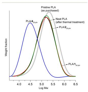
Fig. 5 GPC curves of pristine purchased PLA, neat PLA post thermal treatment under blending conditions, PLA/ $\mathbf{1}_{20~phr}$ , PLA/ $\mathbf{2}_{20~phr}$ , and PLA/ $\mathbf{4}_{20~phr}$ .
