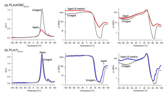
Fig. 8 DMA curves for unaged and aged (6 weeks) specimens of (a) PLA/ATBC $_{20~\mathrm{phr}}$  and (b) PLA/ $1_{20~\mathrm{phr}}$
