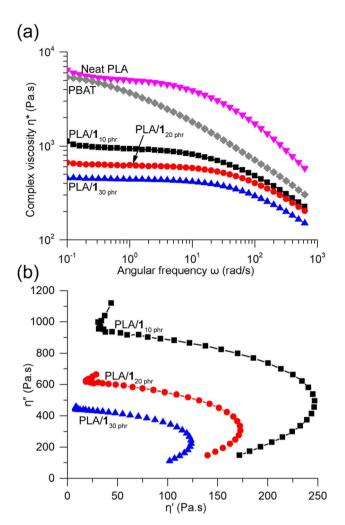
Fig. 7 (a) Dynamic viscosities of PLA/ $\mathbf{1}_{10~phr}$ , PLA/ $\mathbf{1}_{20~phr}$ , and PLA/ $\mathbf{1}_{30~phr}$  compared to neat PLA and PBAT measured using rotational rheometer at 170 °C. (b) Cole–Cole plots of PLA/ $\mathbf{1}_{10~phr}$ , PLA/ $\mathbf{1}_{20~phr}$ , and PLA/ $\mathbf{1}_{30~phr}$ .
