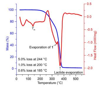
Fig. 6 TGA/DSC analysis of PLA/1<sub>30 phr</sub> blend
