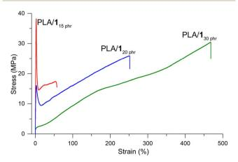
Fig. 3 Stress-strain behavior for PLA/1 blends
