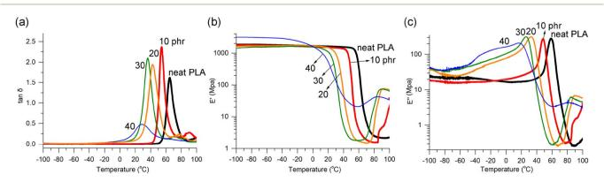
Fig. 2 Temperature dependence of (a)  $\tan \delta$ , (b) storage modulus (E'), (c) loss modulus (E") curves from DMA runs illustrated for PLA/1 blends compared to neat PLA.
