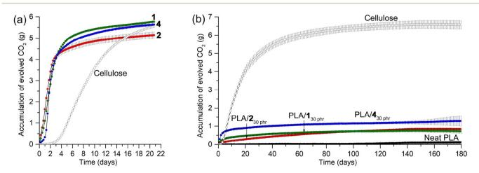
Fig. 9 Biodegradability assessments of (a) organic carbonates and (b) their blends monitored by measuring evolved  $CO_2$  over time in a respirometer set to 25 °C and 50–55% water content with continuous air flow.
