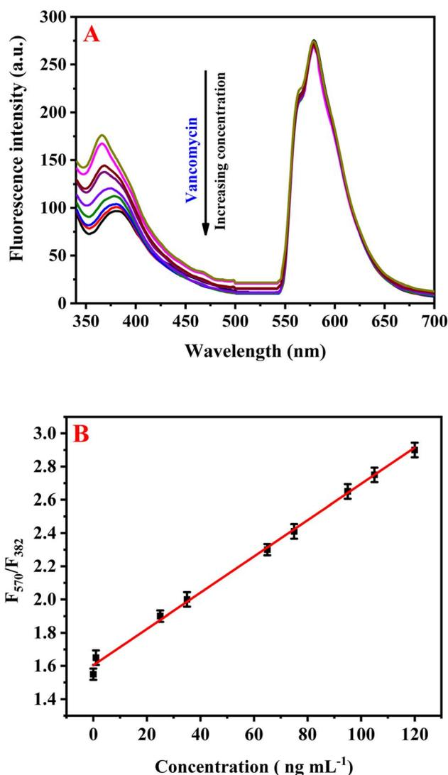
Fig. 3 (A) The effect of different concentrations of vancomycin (0.0–120.0 ng mL<sup>-1</sup>) on the fluorescence intensity of Co@DECDs system. (B) Relationship of ( $F_{570}/F_{382}$ ) versus vancomycin concentrations.
