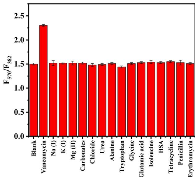
Fig. 4 The effect of different possible interferents (600.0 ng mL<sup>-1</sup>) and vancomycin (65.0 ng mL<sup>-1</sup>) on the fluorescence intensity ratio ( $F_{570}/F_{382}$ ) of Co@DECDs system.
