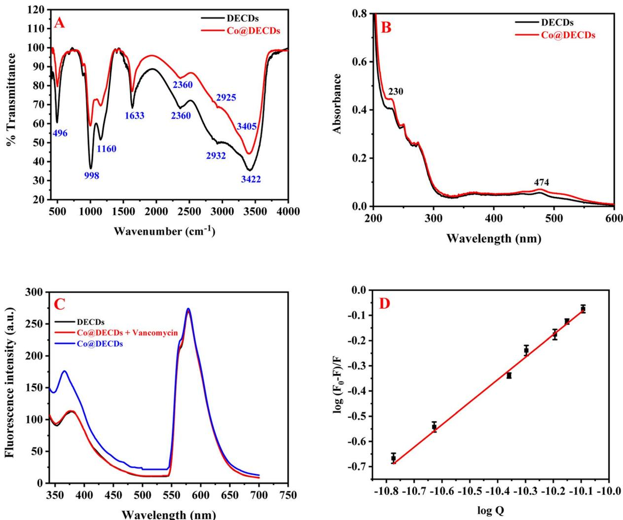
Fig. 5 (A) FT-IR spectral overlay of DECDs and Co@DECDs, (B) UV absorption spectra of DECDs and Co@DECDs, (C) emission spectra overlay of DECDs, Co@DECDs and Co@DECDs + vancomycin (120 ng mL<sup>-1</sup>), (D) plot of  $\log \left[ \frac{F_0 - F}{F} \right]$  versus  $\log [Q]$ .
