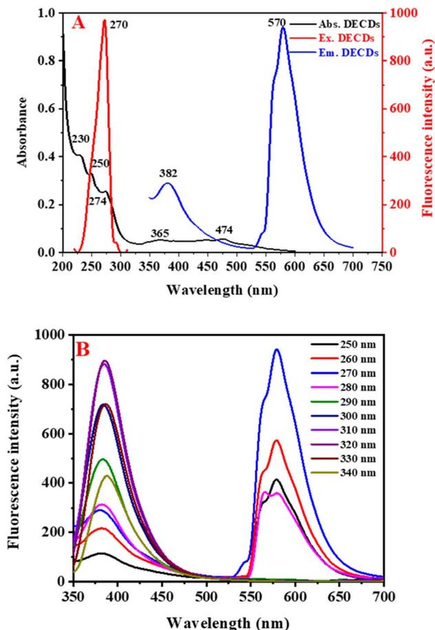
Fig. 2 (A) UV-visible absorption, fluorescence excitation, and emission spectra of the DECDs ( $1.0 \text{ mg mL}^{-1}$ ). (B) Emission spectra of the  $1.0 \text{ mg mL}^{-1}$  DECDs ( $1.0 \text{ mg mL}^{-1}$ ) at excitation wavelengths from 250 to 340 nm.
