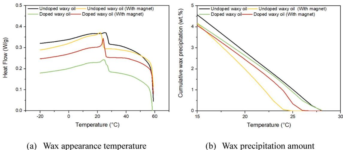
Fig. 9 Wax precipitation properties of the waxy oil under magnetic treatment.
