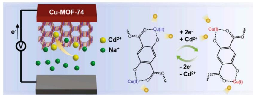
Fig. 10 Schematic representation of the electrochemically assisted capture of cadmium ions. Reproduced with permission from ref. 235 Copyright © 2021, Elsevier.
