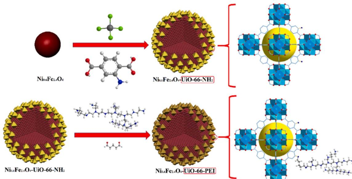
Fig. 6 A schematic showing the procedures to synthesize  $\text{Ni}_{0.6}\text{Fe}_{2.4}\text{O}_4\text{-UiO-66}$ -types. Reproduced with permission from ref. 123 Copyright © 2021, Elsevier.
