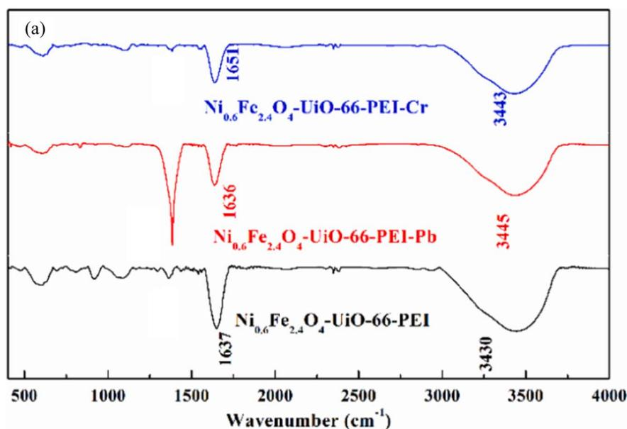
Fig. 7 FTIR spectra of  $\text{Ni}_{0.6}\text{Fe}_{2.4}\text{O}_4\text{-UiO-66-PEI}$  before and after its adsorption of  $\text{Pb(II)}$  or  $\text{Cr(VI)}$  (a). Reproduced with permission from ref. 123 Copyright © 2021, Elsevier.
