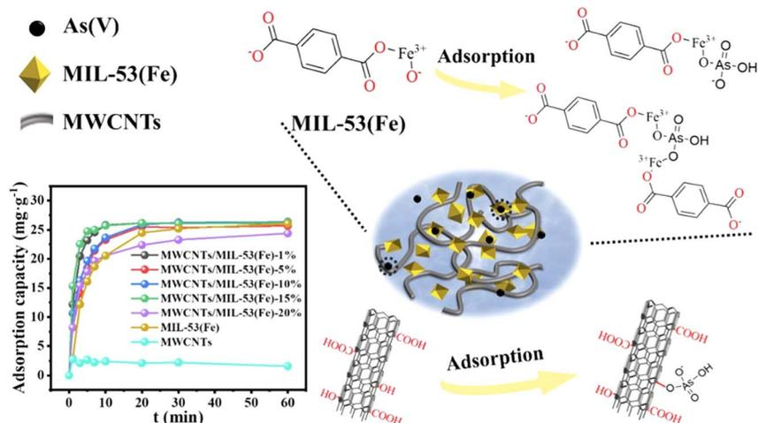
Fig. 12 Schematic of adsorption process and performance of the nanocomposite MWCNTs@MIL-53(Fe) to remove As(v) from polluted water. Reproduced with permission from ref. 278 Copyright © 2023, Elsevier.
