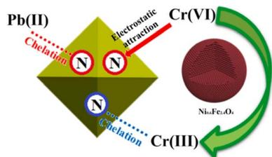
Fig. 8 Adsorption mechanism of  $\text{Ni}_{0.6}\text{Fe}_{2.4}\text{O}_4\text{-UiO-66-PEI}$  for lead and chromium (The N in the circle represents the nitrogen-containing functional group on the surface of  $\text{Ni}_{0.6}\text{Fe}_{2.4}\text{O}_4\text{-UiO-66-PEI}$ ). Reproduced with permission from ref. 123 Copyright © 2021, Elsevier.
