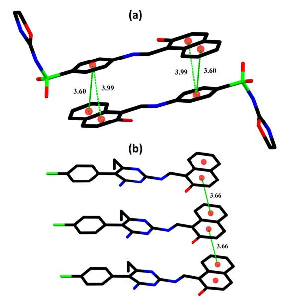
Fig. 3 Graphical representation of the off-set  $\pi \cdots \pi$  stacking interactions in **DSPIN** (a) and **ACPIN** (b). H-atoms not shown for clarity. Distances measured in Å.
