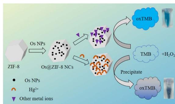
**Scheme 1** Scheme illustration for the Os@ZIF-8 NCs preparation and detection of Hg<sup>2+</sup> concentration.
