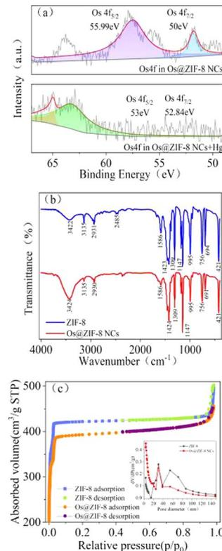
Fig. 2 (a) XPS spectra of the sample in: Os 4f regions of Os@ZIF-8 NCs and Os@ZIF-8 NCs +  $\text{Hg}^{2+}$ , (b) FTIR of ZIF-8 and Os@ZIF-8 NCs, (c)  $\text{N}_2$  sorption isotherms and the pore size distribution plots (inset) of ZIF-8 and Os@ZIF-8 NCs.
