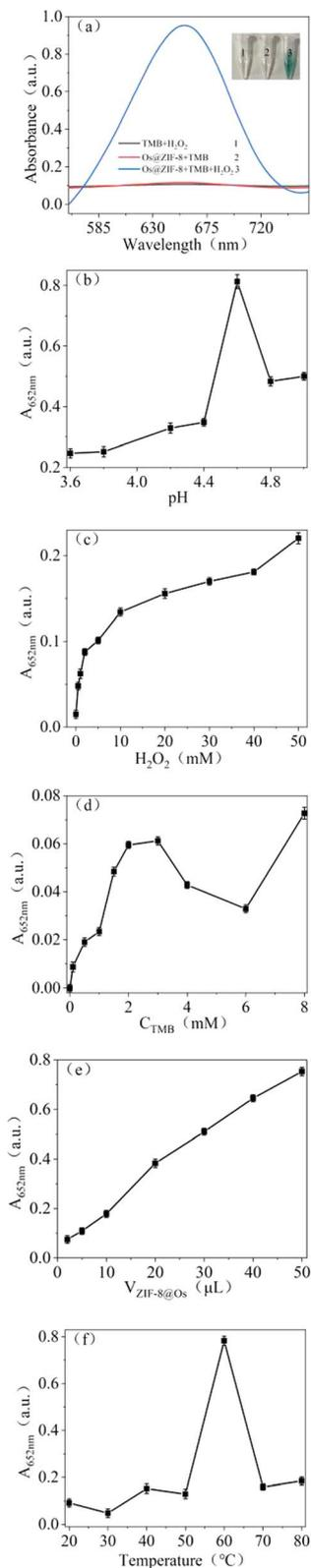
Fig. 3 (a) Absorption spectrum of TMB oxidation in the presence of different substances. Inset is the corresponding images. The effect of experimental conditions on the catalytic activity (b) pH, (c) H<sub>2</sub>O<sub>2</sub> concentration, (d) TMB concentration, (e) the volume of Os@ZIF-8, (f) temperature.
