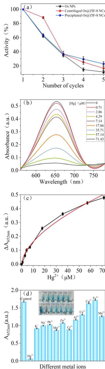
Fig. 6 (a) Activity of pure Os NPs and Os@ZIF-8 NCs in the recycling experiment; (b) UV-vis spectra and (c)  $\Delta A$  at 652 nm with different concentration of  $\text{Hg}^{2+}$  and its linear fitting diagram; (d) absorption values at 652 nm with different metal ions.
