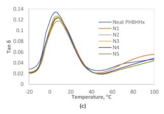
Fig. 9 DMA profiles of Neat PHBHHx and composites: (a) storage modulus, (b) loss modulus, (c)  $\tan\delta$ .
