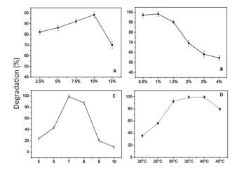
Fig. 10 Effect of: (a) PVA concentration; (b) hectorite concentration; (c) pH; (d) temperature.
