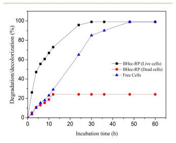
Fig. 6 Decolorization MO using BHec-RP (live and dead cells) and free cells (100 mg  $L^{-1}$ , static, pH 7, temperature 40 °C).
