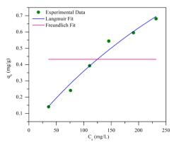
Fig. 8 Non-linear sorption isotherm on BHec-RP (dead cells).
