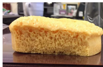
Fig. 16 NIPU foam produced from CLSO and HMDA. Image obtained from ref. 26 with permission from ACS, copyright 2021.
