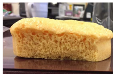
Fig. 16 NIPU foam produced from CLSO and HMDA. Image obtained from ref. 26 with permission from ACS, copyright 2021.
