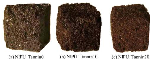
Fig. 27 Images of tannin-glucose-based NIPU foams. Reuse from ref. 157 with permission from Elsevier, copyright 2020.
