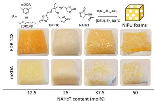
Fig. 26 The effect of NAHcT content on NIPU foaming. Reuse from ref. 156 with permission from ACS, copyright 2022.
