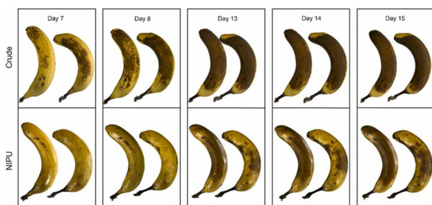
Fig. 30 Experimental study on preservation of bananas using SPR-based NIPU spray coating. Reproduced from ref. 162 with permission from Elsevier, copyright 2022.
