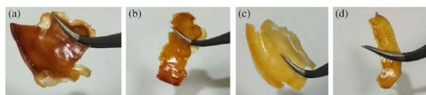
Fig. 11 Physical appearance of NIPU\_1:3 films tested for 48 hours in different media; (a) HCl, (b) NaCl, (c) NaOH, and (d) no chemical environment. Adapted from ref. 88 with permission from Wiley, copyright 2020.
