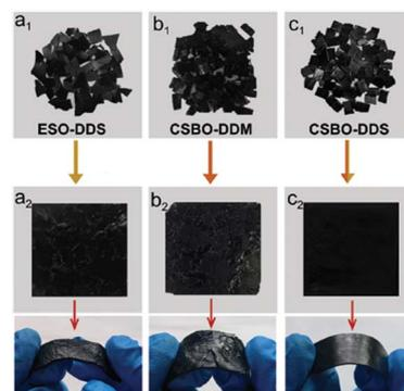
Fig. 13 Reprocessing of (a) single-disulphide ESO-DDS, (b) single carbamate CSBO-DDM, and (c) dual dynamic CSBO-DDS by hot pressing technique. The image obtained from ref. 89 with permission from RSC, copyright 2021.
