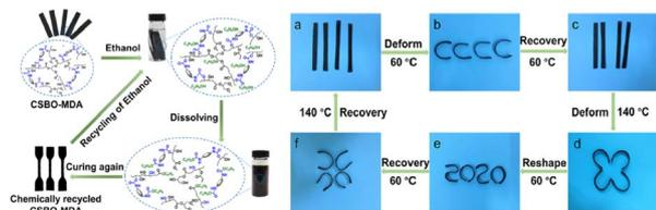
Fig. 14 Chemical recycling process and shape memory effect of CSBO/MDA\_NIPU. (a) deformed at 60 °C and then cooled at 4 °C for a new temporary (b), recovered at 60 °C to the original rectangular shape (c), heated at 140 °C and then cooled at 4 °C (d), reshaped at 60 °C and then cooled at 4 °C shape (e), recovered at 60 °C to the permanent shape (f), and reconfigured at 140 °C to the original shape I. Images obtained from ref. 90 with permission from ACS, copyright 2021.
