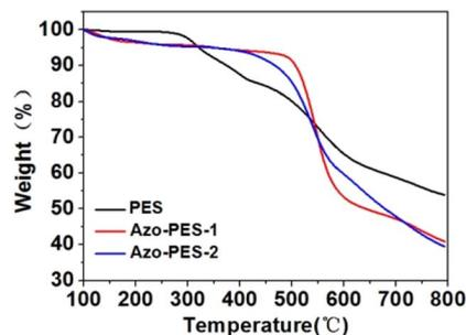
Fig. 7 TGA curves of Azo-PES-1 and Azo-PES-2.
