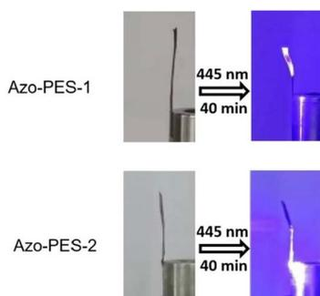
Fig. 11 The photoinduced deformation behavior of the cantilevers under irradiation by a 445 nm laser (100 mW cm<sup>-2</sup>).
