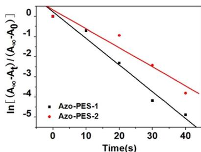
Fig. 6 The first-order *trans*-to-*cis* photoinduced isomerization kinetics of Azo-PES-1 and Azo-PES-2.
