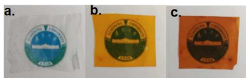
Fig. 9 The transparency of PES (a), Azo-PES-2 (b), and Azo-PES-2 (c) films.
