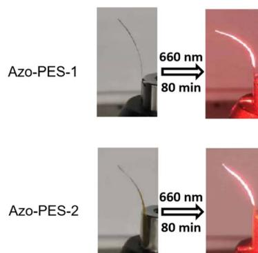
Fig. 13 The photoinduced deformation behavior of the cantilevers under irradiation by a 660 nm laser (100 mW cm<sup>-2</sup>).
