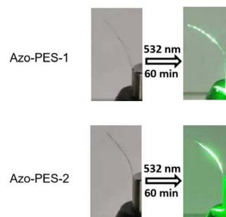
Fig. 12 The photoinduced deformation behavior of the cantilevers under irradiation by a 532 nm laser (100 mW cm<sup>-2</sup>).
