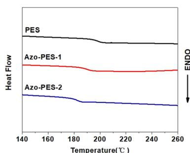
Fig. 8 DSC curves of Azo-PES-1 and Azo-PES-2.
