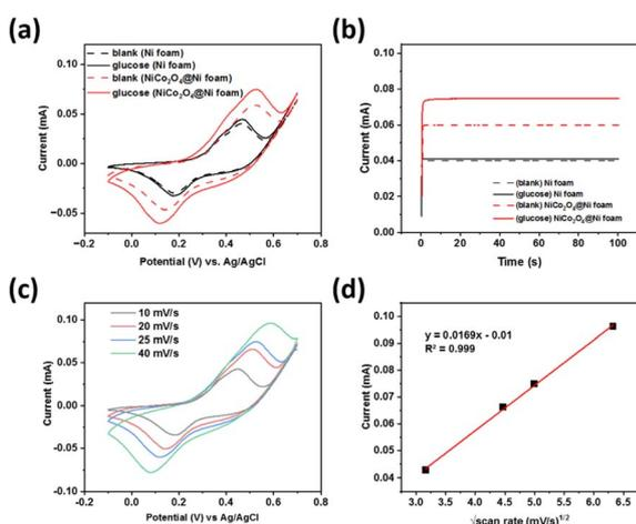
Fig. 6 (a) Cyclic voltammograms at a scan rate of 25 mV s<sup>-1</sup> and (b) chronoamperograms with the prepared NiCo<sub>2</sub>O<sub>4</sub>@Ni foam as the working electrode in comparison with the unmodified Ni foam in 1.0 M NaOH solution with and without the presence of 0.5 μM glucose. (c) Cyclic voltammograms for the prepared NiCo<sub>2</sub>O<sub>4</sub>@Ni foam at various scan rates and (d) the related peak currents plots as a function of the square root of the scan rate.
