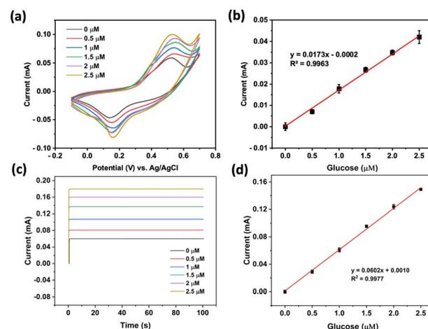
Fig. 7 (a and b) Cyclic voltammograms at a scan rate of 25 mV s<sup>-1</sup> and the related calibration curve, respectively. (c and d) Chronoamperograms at +0.56 V (vs. Ag/AgCl) and the related calibration curve, respectively. The applied working electrode was NiCo<sub>2</sub>O<sub>4</sub>@Ni foam and the electrolytes were various concentrations of glucose in 1.0 M NaOH.
