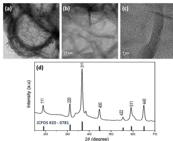
Fig. 3 (a–c) Typical TEM images of the  $\text{NiCo}_2\text{O}_4$  hollow spheres in different magnifications, and (d) XRD spectra for the  $\text{NiCo}_2\text{O}_4$  hollow spheres in comparison with the  $\text{NiCo}_2\text{O}_4$  JCPDS card, shown as the black lines, as the reference.
