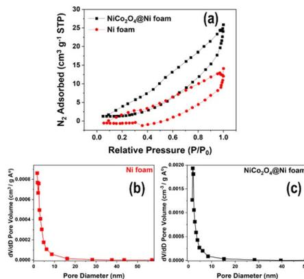
Fig. 5 (a) N<sub>2</sub> adsorption/desorption isotherms of the unmodified Ni foam and the NiCo<sub>2</sub>O<sub>4</sub>@Ni foam; and (b and c) the pore size distributions of the unmodified Ni foam and the NiCo<sub>2</sub>O<sub>4</sub>@Ni foam, respectively.
