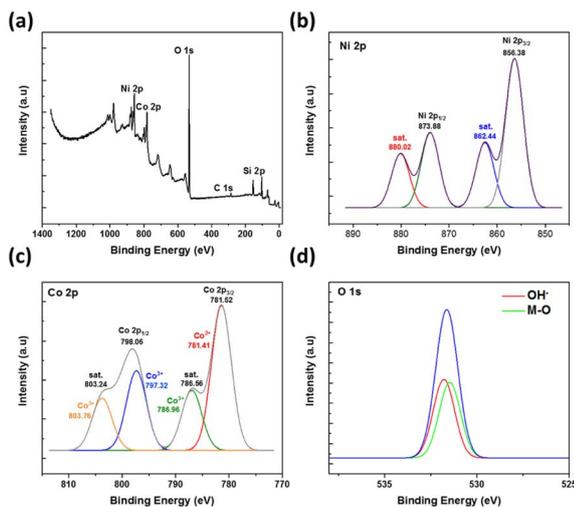
Fig. 4 (a) The XPS spectra of the synthesized NiCo<sub>2</sub>O<sub>4</sub>@Ni foam together with (b–d, respectively) the related deconvolution peaks of Ni 2p, Co 2p, and O 1s.
