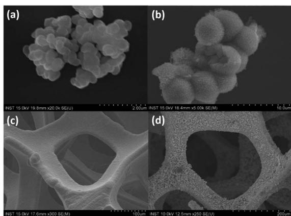
Fig. 2 Typical SEM images of (a) the  $\text{SiO}_2$  nanospheres, (b) the  $\text{NiCo}_2\text{O}_4$  hollow spheres, (c) the unmodified nickel foam, and (d) the  $\text{NiCo}_2\text{O}_4$  hollow spheres deposited on the nickel foam.
