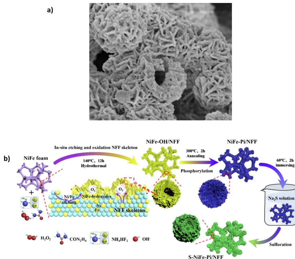
Fig. 12 (a) Mo-NiFe-PO<sub>3</sub>/NFF under SEM magnification, Reproduced from ref. 93 with permission from Elsevier, copyright 2022. (b) S-NiFe-Pi/NFF three-step synthesis procedure, reproduced from ref. 116 with permission from Elsevier, copyright 2023.
