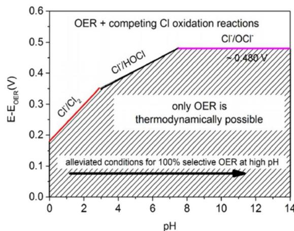
Fig. 4 Maximum permitted overpotentials for OER electrocatalysts, reproduced from ref. 54 with permission from John Wiley and Sons, copyright 2016.<sup>54</sup>
