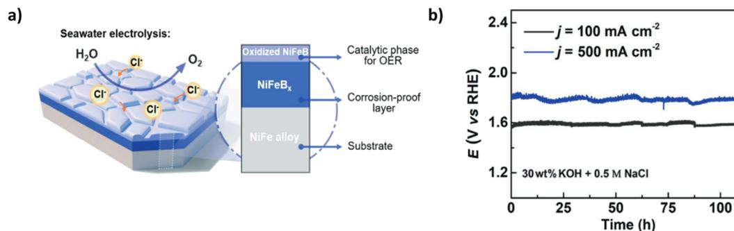
Fig. 13 (a) Schematic of NiFeB<sub>x</sub> electrode with a breakdown of relevant layers (b) chronopotentiometry curve of NiFeB<sub>x</sub> electrode in simulated seawater at 100 and 500 mA cm<sup>-2</sup>. Reproduced from ref. 96 with permission from John Wiley and Sons, copyright 2021.
