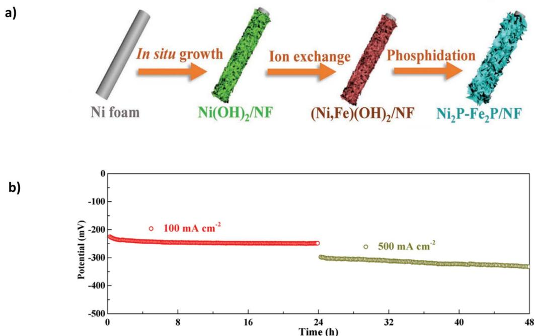
Fig. 11 (a) Ni<sub>2</sub>P-Fe<sub>2</sub>P/NF three-step synthesis method. (b) Stability of Ni<sub>2</sub>P-Fe<sub>2</sub>P/NF in 1 M KOH + seawater at 100 mA cm<sup>-2</sup> and 500 mA cm<sup>-2</sup>. Reproduced from ref. 91 with permission from John Wiley and Sons, copyright 2020.
