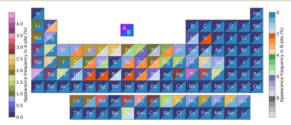
Fig. 13 The appearance frequency of the A- and B-site elements of the 682 143 predicted stable perovskites oxides with  $E_h$  values of lower than 50 meV atom<sup>-1</sup>.
