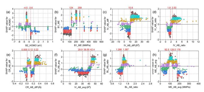
Fig. 8 SHAP dependence plots of the top eight features for perovskite stability prediction: (a) B2\_HOMO, (b) B1\_ME, (c) IV\_AB\_diff, (d) IV\_AB\_ratio, (e) CR\_AB\_diff, (f) IV\_AB\_avg, (g) BL\_AB\_ratio, (h) ME\_AB\_avg.
