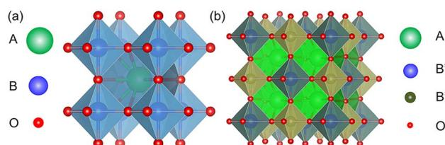
Fig. 1 Structure diagrams of (a) single and (b) double perovskite oxides.<sup>11</sup>
