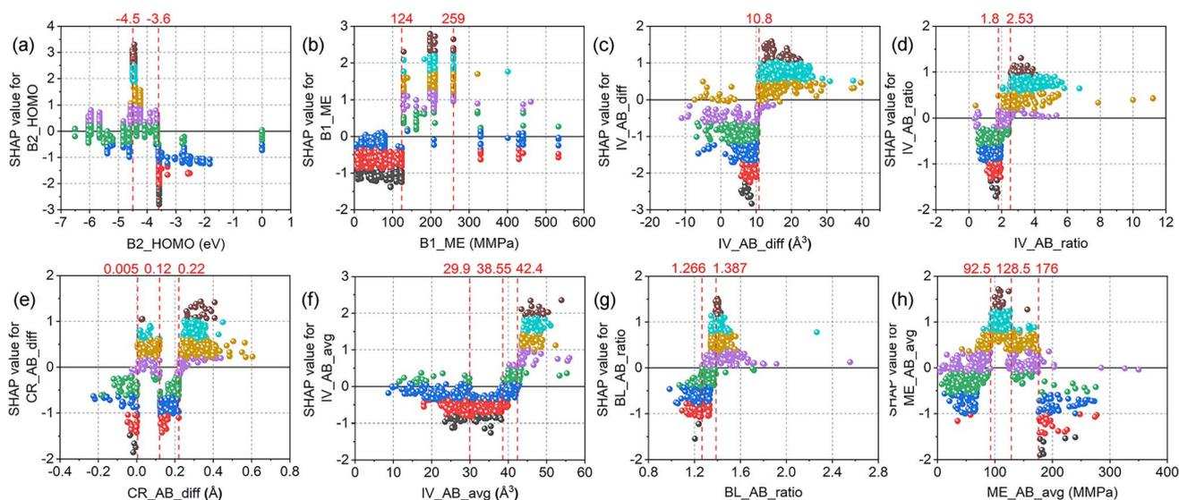
Fig. 8 SHAP dependence plots of the top eight features for perovskite stability prediction: (a) B2\_HOMO, (b) B1\_ME, (c) IV\_AB\_diff, (d) IV\_AB\_ratio, (e) CR\_AB\_diff, (f) IV\_AB\_avg, (g) BL\_AB\_ratio, (h) ME\_AB\_avg.
