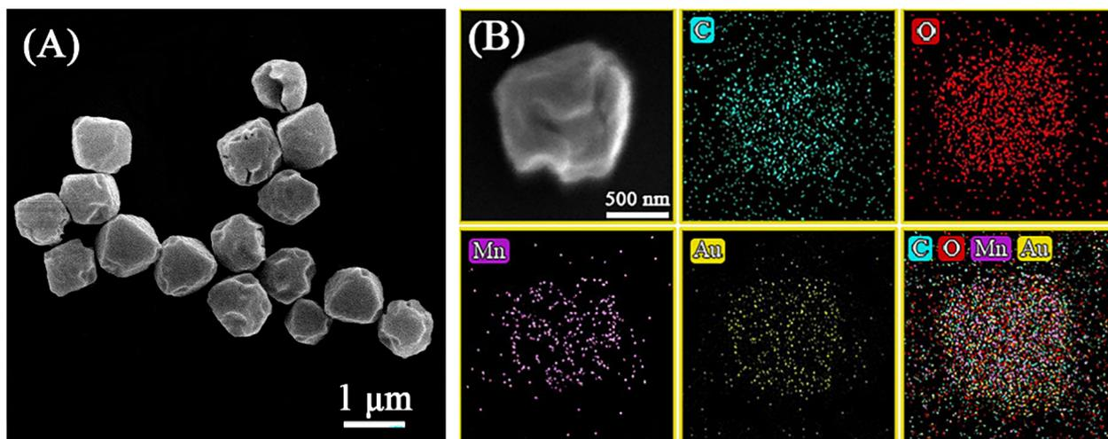
Fig. 1 (A) SEM image, and (B) element distributions of C, O, Mn and Au species *via* SEM-EDX of Au/Mn-MIL-100.
