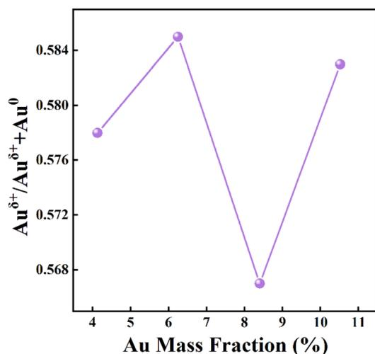
**Fig. 6** The influence of Au mass fraction on the Au<sup>δ+</sup>/(Au<sup>δ+</sup> + Au<sup>δ0</sup>) molar ratio of the Au<sub>x</sub>/Mn<sub>3</sub>O<sub>4</sub> catalysts.
