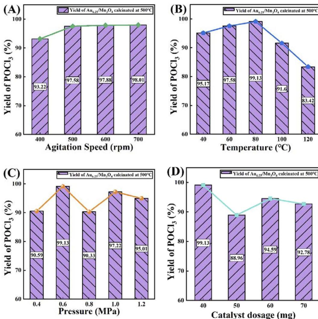
Fig. 8 The influence of (A) agitation speed, (B) reaction temperature, (C) reaction pressure and (D) catalyst dosage on catalytic performance of  $\text{Au}_{6.25}/\text{Mn}_3\text{O}_4$  in terms of the yield of  $\text{POCl}_3$  in the  $\text{PCl}_3$  oxidation reaction.
