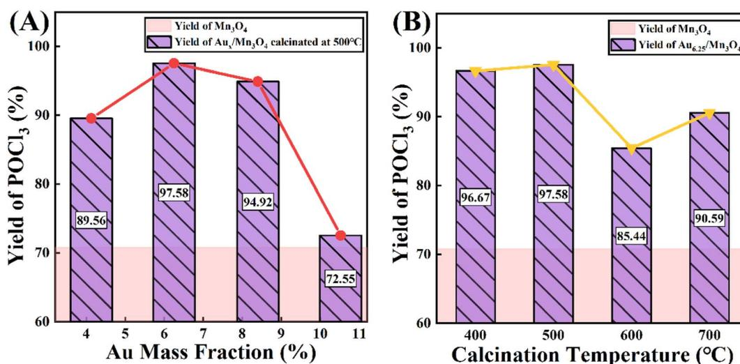
**Fig. 7** The influence of (A) Au mass fraction and (B) calcination temperature on catalytic performance of Au/Mn<sub>3</sub>O<sub>4</sub> in terms of the yield of POCl<sub>3</sub> in the PCl<sub>3</sub> oxidation reaction.
