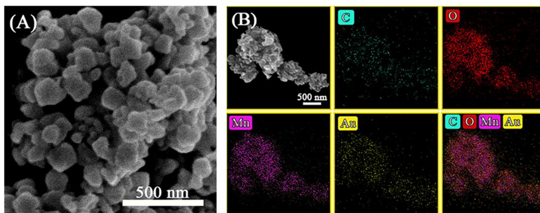
Fig. 4 (A) SEM image, and (B) element distribution of C, O, Mn and Au species *via* SEM-EDX of Au <sub>$x$</sub> /Mn<sub>3</sub>O<sub>4</sub>.
