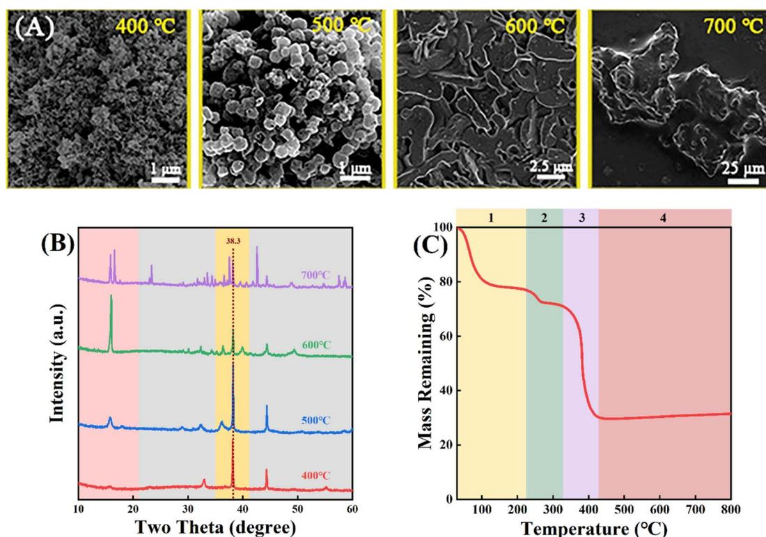
Fig. 3 (A) SEM images and (B) XRD patterns of Au<sub>2</sub>/Mn-MIL-100 calcined at different temperatures (400, 500, 600 and 700 °C) under air. (C) Weight loss of Au<sub>2</sub>/Mn-MIL-100 calcined under air.
