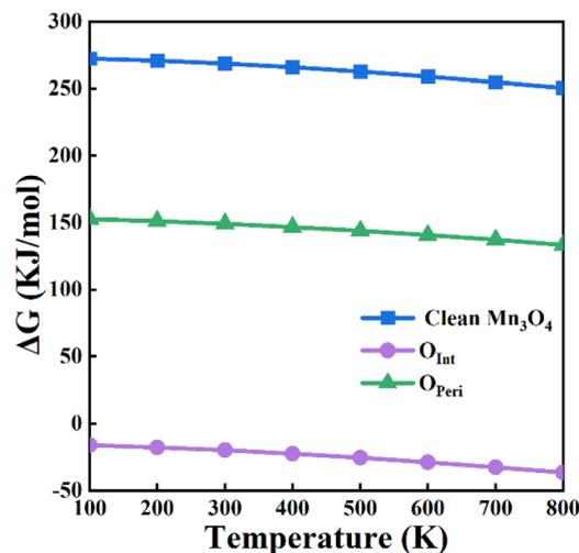
Fig. 10 Variation in  $\Delta G$  for the formation of  $\text{POCl}_3$  using the lattice oxygens of  $\text{Mn}_3\text{O}_4$  and using the interface and perimeter lattice oxygens of the  $\text{Au}_{10}/\text{Mn}_3\text{O}_4$  model system.
