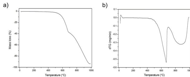
Fig. 3 TG (a) and DTG (b) diagrams for graphite-PbCl<sub>2</sub>-FeCl<sub>3</sub> composite.
