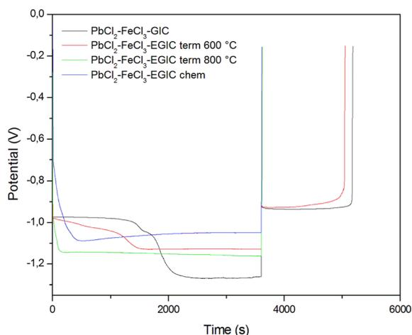
Fig. 7 Galvanostatic curves recorded for the examined composites in 1 M H<sub>2</sub>SO<sub>4</sub> water solution.
