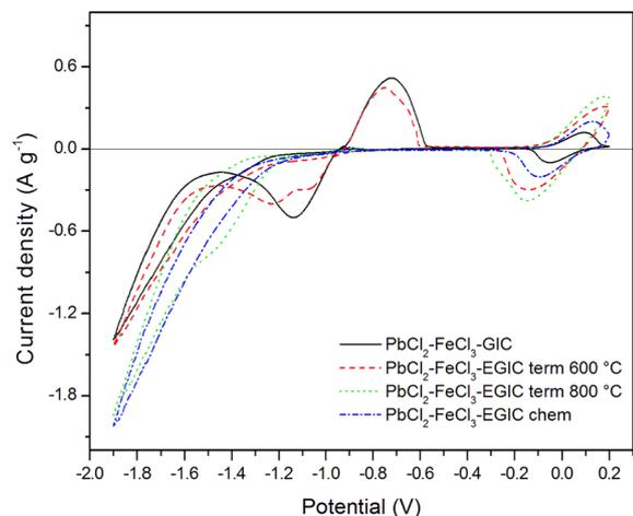
Fig. 5 Cyclic voltammograms recorded for the examined composites in 1 M H<sub>2</sub>SO<sub>4</sub> water solution in the potential range from -1.9 V to 0.2 V. Scan rate 10 mV s<sup>-1</sup>.
