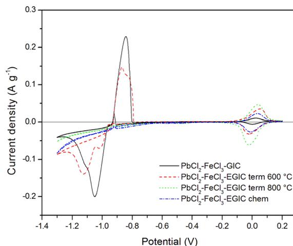
Fig. 6 Cyclic voltammograms recorded for the examined composites in 1 M H<sub>2</sub>SO<sub>4</sub> water solution in the potential range from -1.3 V to 0.2 V. Scan rate 1 mV s<sup>-1</sup>.
