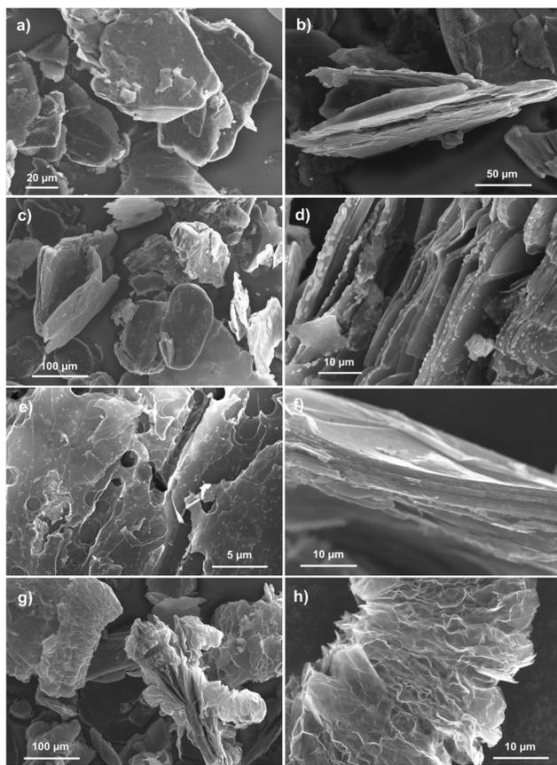
Fig. 1 SEM images of the original graphite–PbCl<sub>2</sub>–FeCl<sub>3</sub> composite (a and b), graphite–PbCl<sub>2</sub>–FeCl<sub>3</sub> composite heat treated at 600 °C (c and d) and 800 °C (e and f), chemically modified graphite–PbCl<sub>2</sub>–FeCl<sub>3</sub>-composite (g and h).
