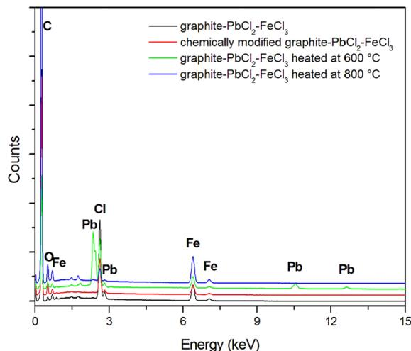
Fig. 2 EDS spectra for the examined composites.
