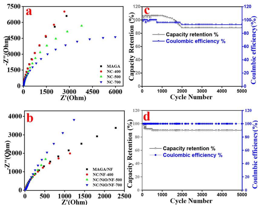
Fig. 9 (a and b) Nyquist plots and (c and d) cycling stability for (a), (c) NC-400 and (b and d) NC/NF-400 at  $10 \text{ A g}^{-1}$ .
