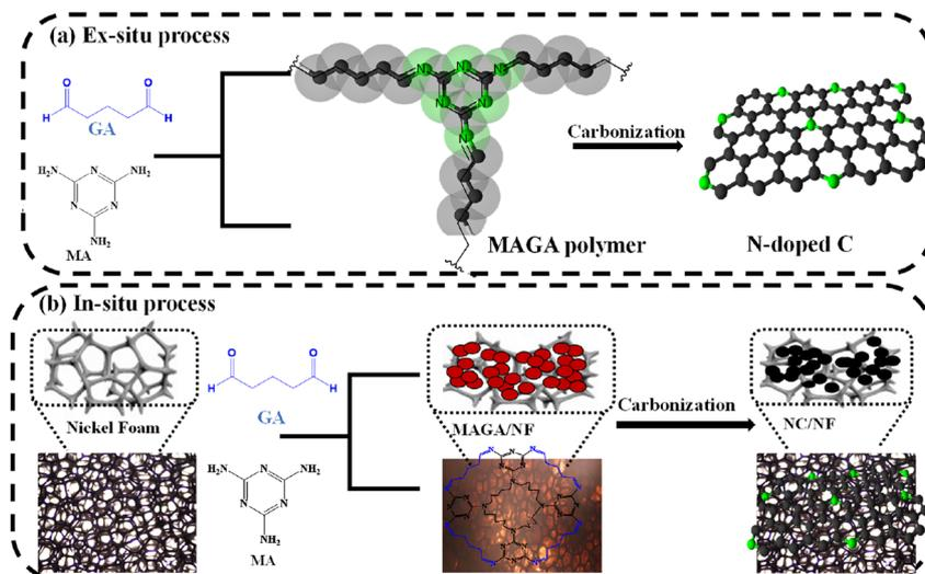
Fig. 1 The formation of MAGA and their carbonization into NC using (a) *ex situ* and (b) *in situ* processes.
