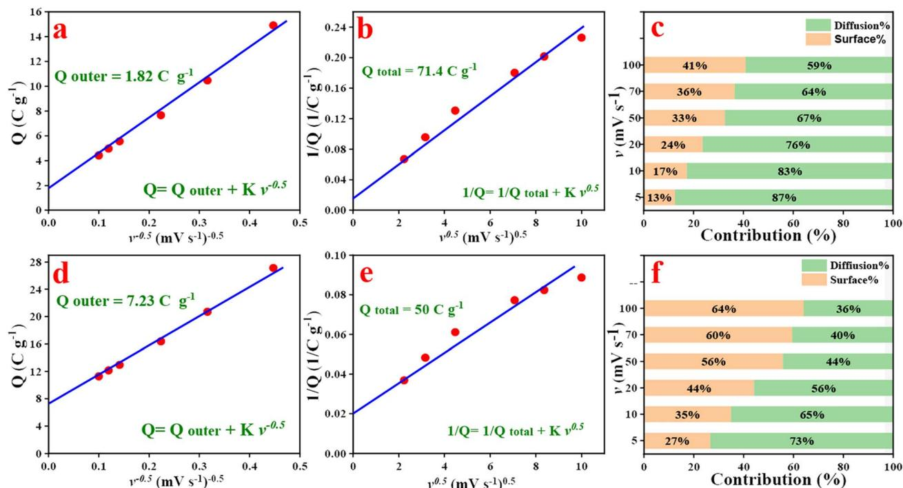
Fig. 6 Relation between  $Q$  vs.  $v^{-0.5}$  (a–d),  $1/Q$  vs.  $v^{0.5}$  (b–e), and (c–f) bar graph of surface and diffusion contributions at different scan rates of carbonized materials at 400 °C using (a–c) *in situ* and (d–f) *ex situ* processes.
