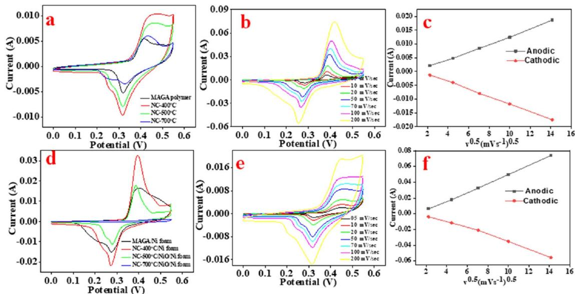
Fig. 5 CV curves for electrode materials synthesized *via* (a–c) *ex situ* and (d–f) *in situ* procedure, (c and f) the linear relationship between  $I$  and  $v^{0.5}$  of the carbonized electrode at 400 °C prepared by (c) *ex situ* and (f) *in situ* process.
