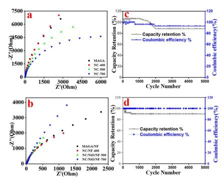
Fig. 9 (a and b) Nyquist plots and (c and d) cycling stability for (a), (c) NC-400 and (b and d) NC/NF-400 at 10 A  $g^{-1}$ .
