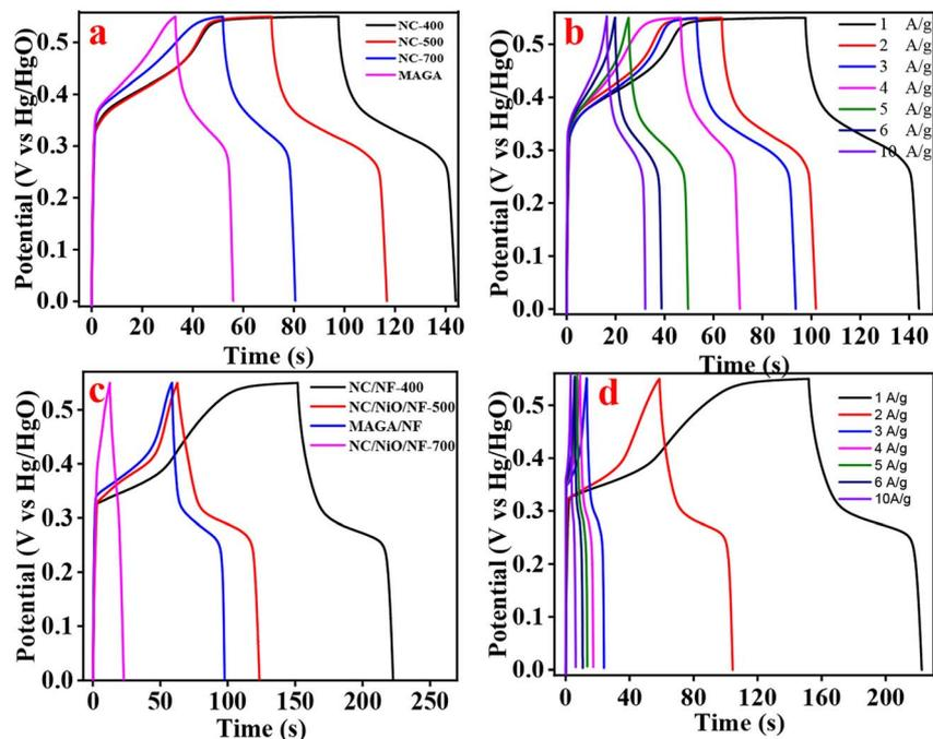
Fig. 7 GCD curves for electrodes prepared via (a) *ex situ* and (c) *in situ* procedure at  $1 \text{ A g}^{-1}$  and GCD curves at different current densities from 1–10  $\text{A g}^{-1}$  (b) NC-400 and (d) NC/NF-400.
