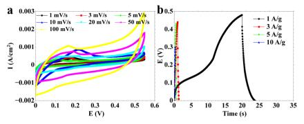
Fig. 10 Electrochemical measurements of two electrode systems using a symmetric device via (a) CV curves and (b) GCDC.
