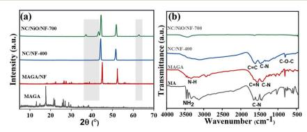
Fig. 2 Electrode and MAGA powder characterization using (a) XRD and (b) FT-IR spectra.
