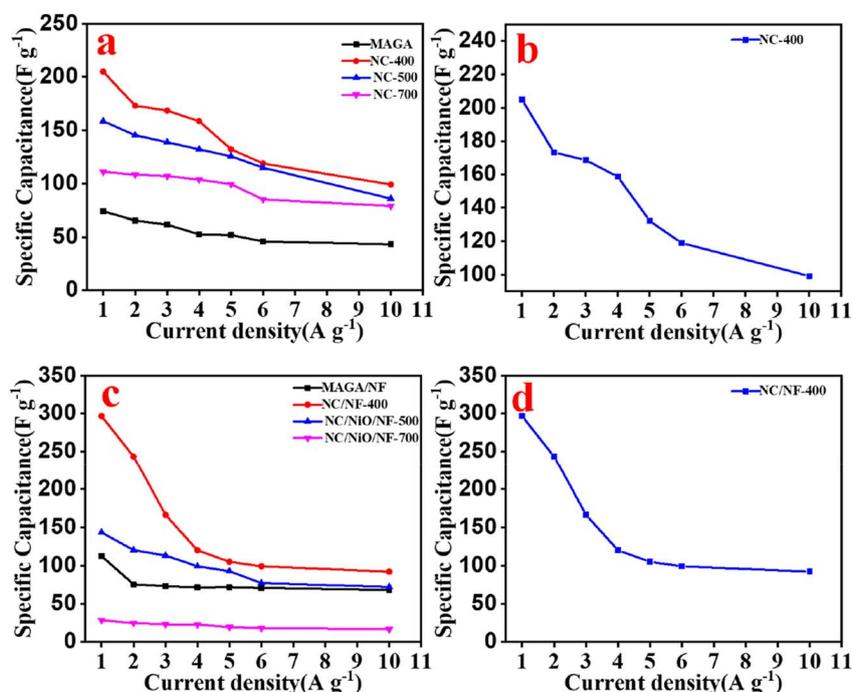
Fig. 8 (a–c) Specific capacitance for all electrodes prepared by *ex situ* and *in situ* processes at different current densities, specific capacitance of (b) NC-400 and (d) NC/NF-400 at a different current density.
