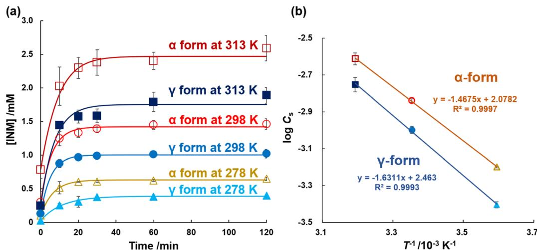
Fig. 4 (a) INM dissolution behaviors in 25 mM  $\text{KH}_2\text{PO}_4/\text{Na}_2\text{HPO}_4$  buffer at pH 6.8 ( $n = 3$ );  $\alpha$ -form at 313 K (open squares),  $\gamma$ -form at 313 K (closed squares),  $\alpha$ -form at 298 K (open circles),  $\gamma$ -form at 298 K (closed circles),  $\alpha$ -form at 278 K (open triangles),  $\gamma$ -form at 278 K (closed circles). (b) Van't Hoff plots of INM;  $\alpha$ -form (circles) and  $\gamma$ -form (squares).
