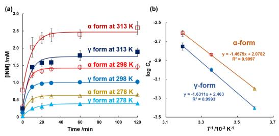
Fig. 4 (a) INM dissolution behaviors in 25 mM KH<sub>2</sub>PO<sub>4</sub>/Na<sub>2</sub>HPO<sub>4</sub> buffer at pH 6.8 (n=3);  $\alpha$ -form at 313 K (open squares),  $\gamma$ -form at 313 K (closed squares),  $\alpha$ -form at 298 K (open circles),  $\gamma$ -form at 298 K (closed circles),  $\alpha$ -form at 278 K (open triangles),  $\gamma$ -form at 278 K (closed circles). (b) Van't Hoff plots of INM;  $\alpha$ -form (circles) and  $\gamma$ -form (squares).
