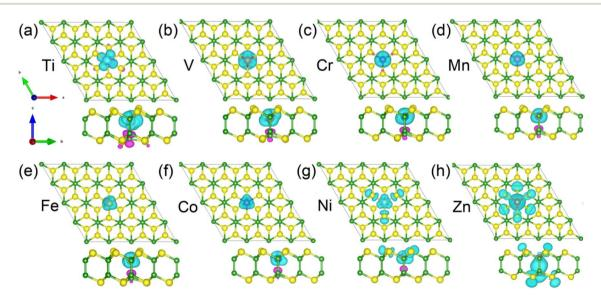
Fig. 4 (a-h) The spin density distribution of 3d-TM doped B<sub>2</sub>S<sub>2</sub> monolayers with 3.12% doping from both the top and the side view. Isovalue is 0.02 eV Å<sup>-3</sup>. The spin-up and spin-down densities are represented by the sky blue and purple isosurfaces, respectively.
