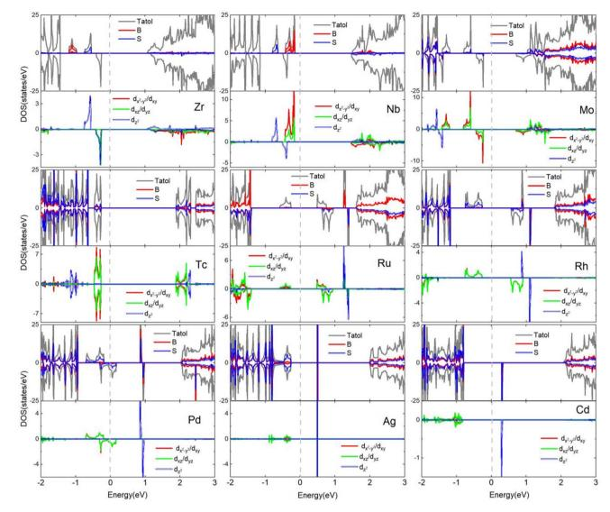
Fig. 7 The total and projected density of states of 4d-TM doped  $B_2S_2$  monolayers with 3.12% doping. The Fermi energy is shifted to zero energy as indicated by the vertical dashed black line.
