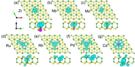
Fig. 6 (a–g) The calculated spin densities of 4d-TM doped  $B_2S_2$  monolayers with 3.12% doping from both the top view and the side view. Isovalue is 0.02 eV Å<sup>-3</sup>. The spin-up and spin-down densities are represented by the sky blue and purple isosurfaces, respectively.
