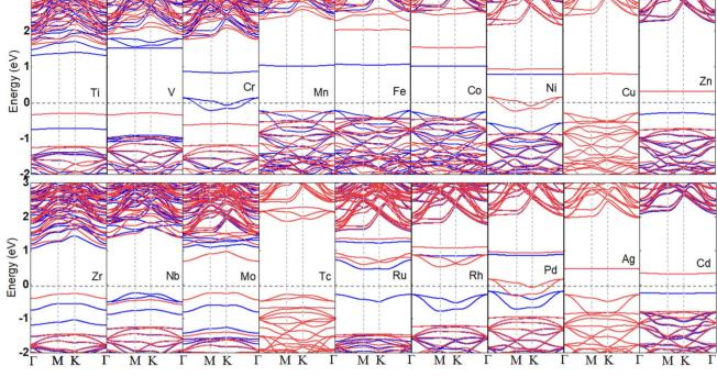
Fig. 3 The calculated band structures of a 3d- and 4d-TM doped B<sub>2</sub>S<sub>2</sub> monolayers with 3.12% doping. The spin-up and spin-down states are represented by the blue and red lines, respectively. The zero of the energy is set to the Fermi level, shown by the grey lines.
