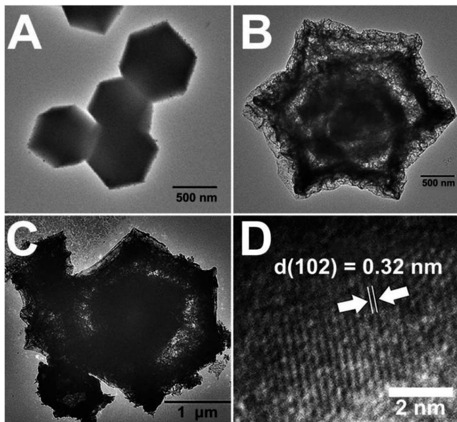
Fig. 1 TEM images of (A) ZIF-67, (B) Co<sub>3</sub>O<sub>4</sub>, and (C) Co<sub>3</sub>O<sub>4</sub>/90.0 wt% AZIS. (D) HRTEM image of the Co<sub>3</sub>O<sub>4</sub>/90.0 wt% AZIS.
