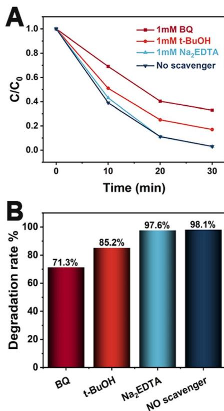
Fig. 6 (A) Variation trend in MO concentration over time in the presence of  $\text{Co}_3\text{O}_4/90.0$  wt% AZIS and three different scavengers (B) the corresponding summaries of degradation percentage after 30 min irradiation.
