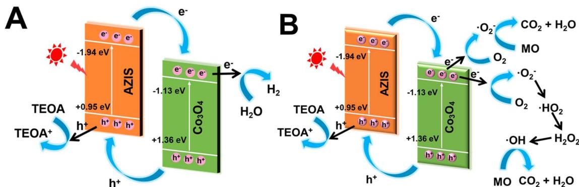
Scheme 2 Schematic illustration of the possible mechanisms for (A) the photocatalytic  $\text{H}_2$  production and (B) the MO degradation on the dodecahedral HoMs  $\text{Co}_3\text{O}_4/\text{AZIS}$  photocatalyst under visible light irradiation.
