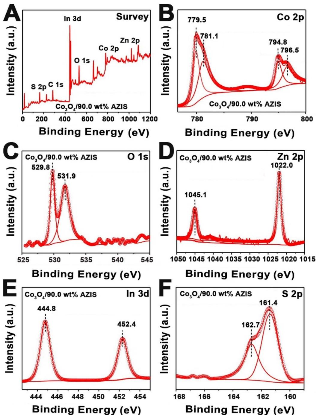
Fig. 3 XPS spectrum of  $\text{Co}_3\text{O}_4/90.0 \text{ wt\% AZIS}$ : (A) survey spectrum, and (B) Co 2p, (C) O 1s, (D) Zn 2p, (E) In 3d, and (F) S 2p high-resolution spectra.
