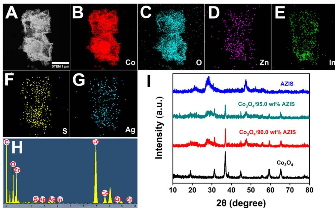
Fig. 2 (A) HAADF-STEM image of Co<sub>3</sub>O<sub>4</sub>/90.0 wt% AZIS, (B–G) the corresponding elemental mapping images of Co, O, Zn, In, S, and Ag elements, and (H) the corresponding EDX spectrum. (I) XRD patterns of Co<sub>3</sub>O<sub>4</sub>, AZIS, and Co<sub>3</sub>O<sub>4</sub>/AZIS.
