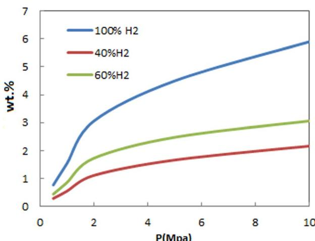
Fig. 8 Comparison of hydrogen adsorption isotherms of FeCNT at 298 K from pure H<sub>2</sub> and H<sub>2</sub>/N<sub>2</sub> mixture.
