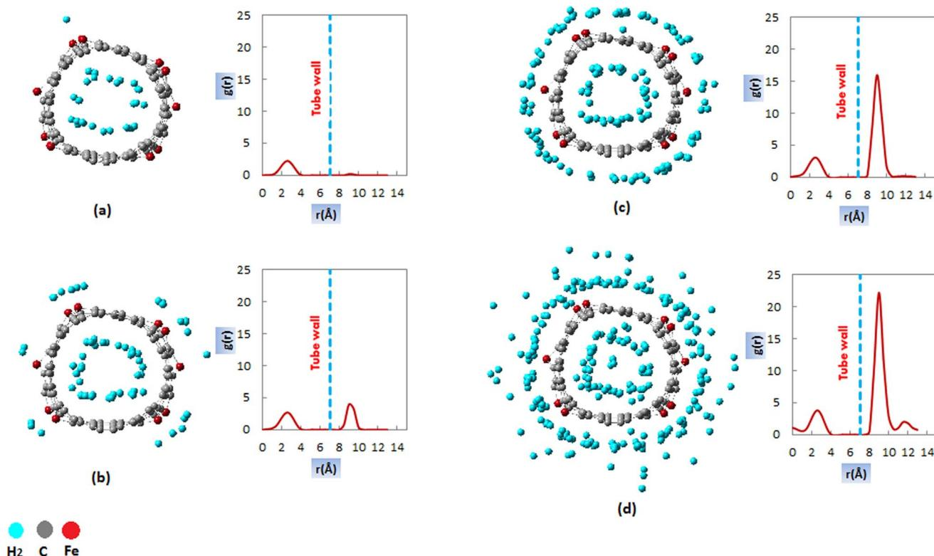
Fig. 5 Radial distribution functions of H<sub>2</sub> molecules inside and outside the FeCNT versus distance from the central axis of the nanotube and Snapshot generated by the simulation of hydrogen storage at 298 K and (a) 1 MPa (b) 2 MPa (c) 5 MPa (d) 10 MPa.
