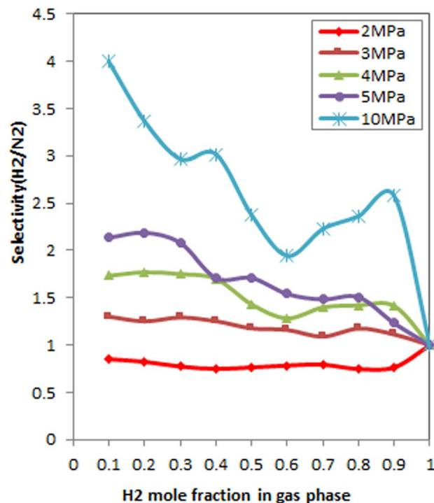
Fig. 10 Selectivity of H<sub>2</sub>/N<sub>2</sub> as a function of H<sub>2</sub> bulk composition at 298 K and different pressures.
