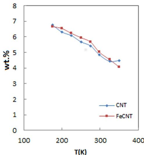
Fig. 7 Variation of H<sub>2</sub> adsorption capacity of FeCNT and pure CNT upon the temperature increment at 5 MPa.
