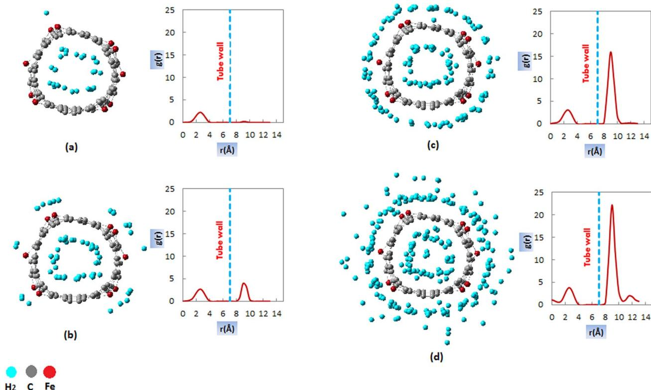
Fig. 5 Radial distribution functions of  $\text{H}_2$  molecules inside and outside the FeCNT *versus* distance from the central axis of the nanotube and Snapshot generated by the simulation of hydrogen storage at 298 K and (a) 1 MPa (b) 2 MPa (c) 5 MPa (d) 10 MPa.
