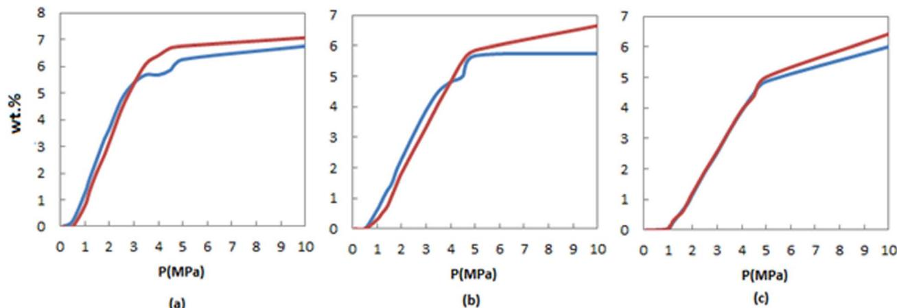
Fig. 4 Comparison of  $\text{H}_2$  adsorption isotherms of FeCNT (red line) and pure CNT (blue line) at (a) 175, (b) 250 and (c) 298 K.
