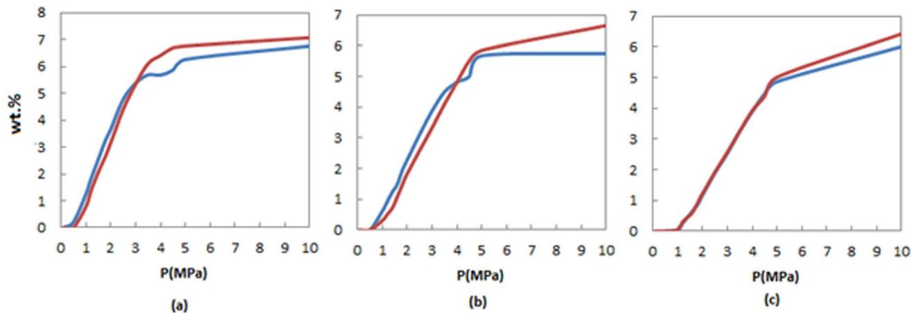
Fig. 4 Comparison of H<sub>2</sub> adsorption isotherms of FeCNT (red line) and pure CNT (blue line) at (a) 175, (b) 250 and (c) 298 K.
