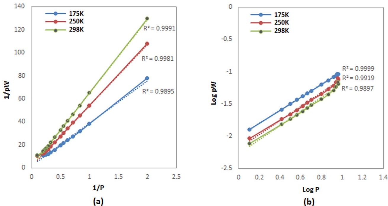
Fig. 6 Fitting isotherms plots for H<sub>2</sub> adsorption at different temperatures (a) Langmuir (b) Freundlich.
