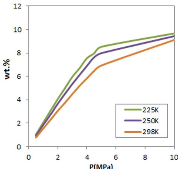
Fig. 3 Total  $\text{H}_2$  adsorption isotherms of FeCNT at 225, 250 and 298 K.
