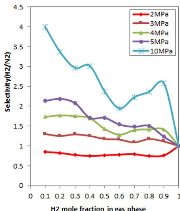
Fig. 10 Selectivity of H<sub>2</sub>/N<sub>2</sub> as a function of H<sub>2</sub> bulk composition at 298 K and different pressures.
