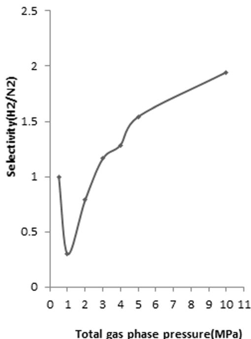
Fig. 9 H<sub>2</sub> selectivity of FeCNT from mixture of 60 mol% H<sub>2</sub>/N<sub>2</sub> vs. pressure at 298 K (mole fraction of 0.6 H<sub>2</sub> and 0.4 N<sub>2</sub> mixtures).
