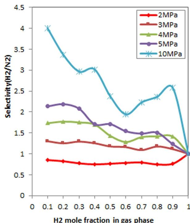
Fig. 10 Selectivity of H<sub>2</sub>/N<sub>2</sub> as a function of H<sub>2</sub> bulk composition at 298 K and different pressures.
