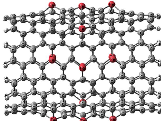
Fig. 1 Optimized structure of FeCNT.
