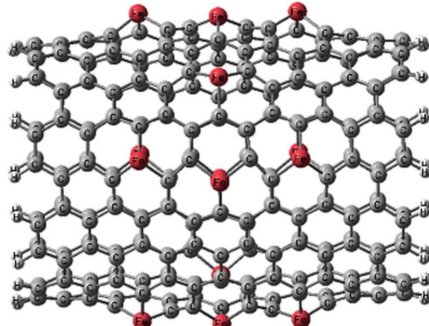
Fig. 1 Optimized structure of FeCNT.
