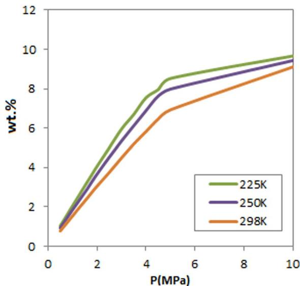
Fig. 3 Total H<sub>2</sub> adsorption isotherms of FeCNT at 225, 250 and 298 K.
