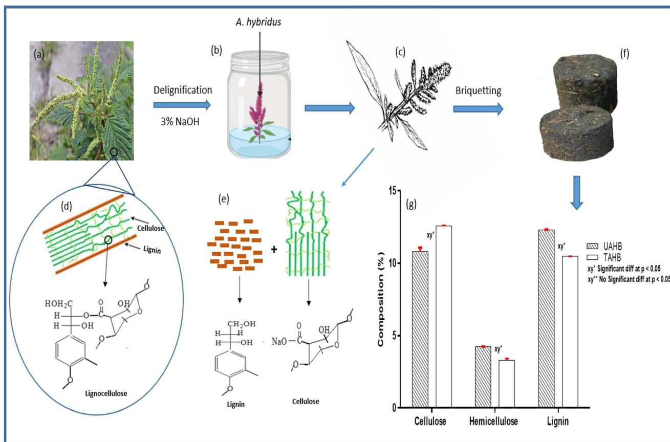
Fig. 2 The scheme showing (a) Fresh *Amaranthus hybridus* plant (b) delignification of the fiber matrix of untreated *Amaranthus hybridus* (c) dried *Amaranthus hybridus* waste (d) delignification of lignocellulose (e) disrupted lignocellulose to lignin and cellulose (f) treated *Amaranthus hybridus* briquettes and (g) lignocellulose composition of treated *Amaranthus hybridus* briquettes.
