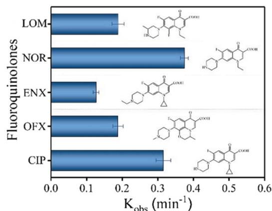
Fig. 21 Kinetic rate constants of 2BNRU for fluoroquinolones when exposed to visible light.<sup>201</sup>
