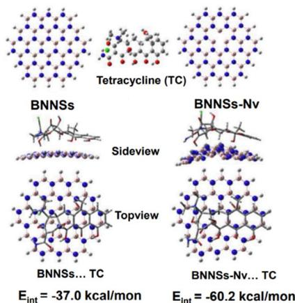
Fig. 16 Best possible structures of BN nanosheets (BNNs) and N-defective BNNs with N vacancy (BNNs-Nv) and their related adsorbed forms.<sup>170</sup>
