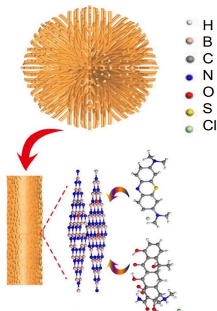
Fig. 15 Sea urchin-like hexagonal BN's potential adsorption mechanism diagram for methylene blue and tetracycline.<sup>169</sup>
