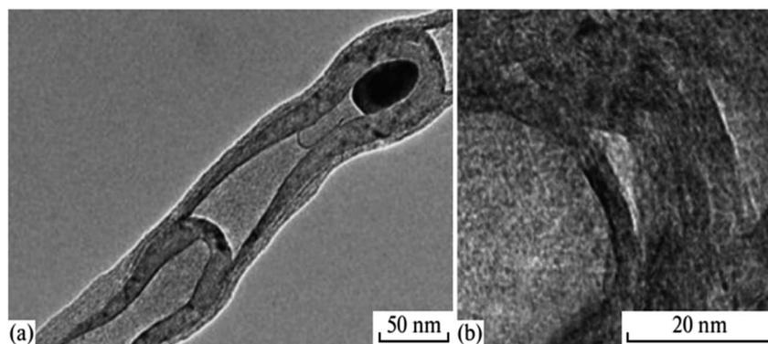
Fig. 6 (a) TEM image and (b) HRTEM image of a bamboo-like nanotube.<sup>56</sup>
