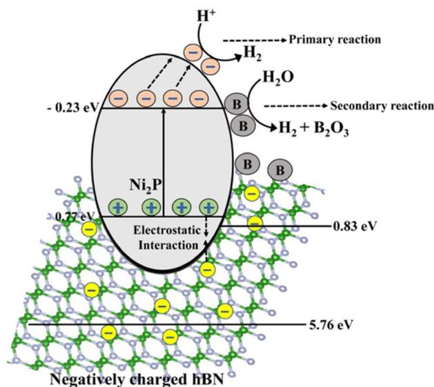
**Fig. 25** The schematic illustration of the mechanism of the photocatalytic H<sub>2</sub> production by the B/h-BN/Ni<sub>2</sub>P nanocomposite.<sup>283</sup>
