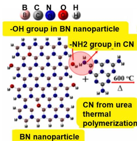
Fig. 14 The layered BN-carbon nitride composites (BN-30-600) are thought to be generated using urea and BN nanoparticles as precursors.<sup>137</sup>
