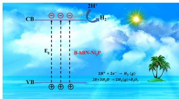
**Fig. 24** Water splitting via photocatalytic hydrogen evolution.<sup>274</sup>
