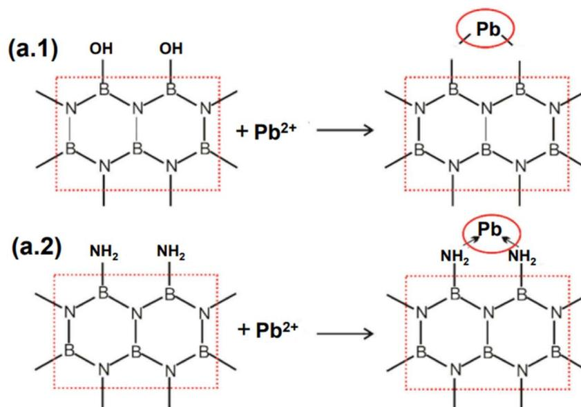
Fig. 13 The probable mechanisms of (a.1) B–OH & (a.2)  $-\text{NH}_2$  in lead ion adsorption on the BN-550 nanostructure.<sup>113</sup>
