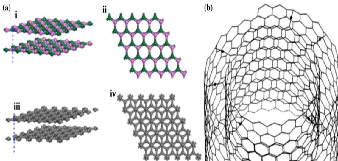
Fig. 2 (a) Morphology of (i) and (ii) h-BN sheets and (iii) and (iv) graphite sheets showing differences in the order in which they are stacked.<sup>31</sup> (b) Interaction between the neighbouring layers of a multi-walled nanotube.<sup>32</sup>
