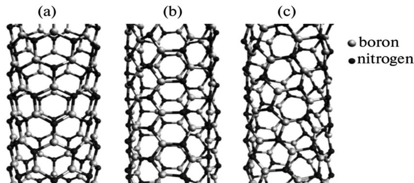
Fig. 5 Simulation of various chiralities in BN nanotubes: (a) zigzag, (b) armchair, and (c) chiral configurations.<sup>56</sup>
