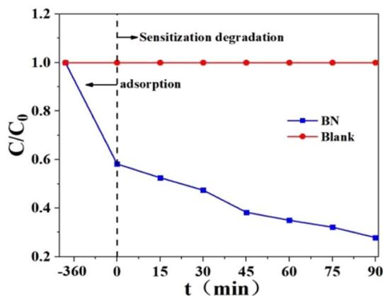
Fig. 22 Rh-B elimination by BN under vis-light irradiation.<sup>240</sup>
