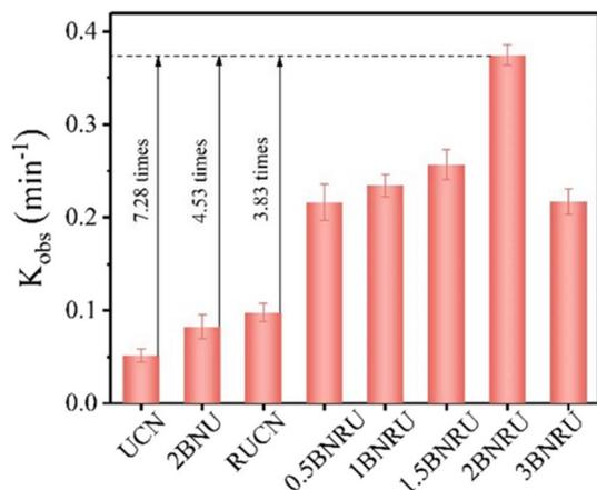
Fig. 19 Kinetic rate constant based on the photocatalytic activity.<sup>203</sup>
