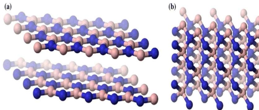
Fig. 1 Crystal form of (a) hexagonal boron nitride and (b) cubic boron nitride.<sup>25</sup>
