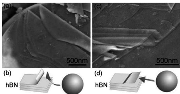
Fig. 9 SEM images illustrating the mechanism of mechanical exfoliation; (a) and (b) cleavage at the edge of h-BN nanoparticles, and (c) and (d) peeling of h-BN thin sheets by ball milling.<sup>65</sup>
