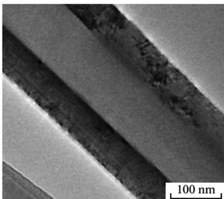
Fig. 7 TEM image of a multiwall BN nanotube.<sup>56</sup>
