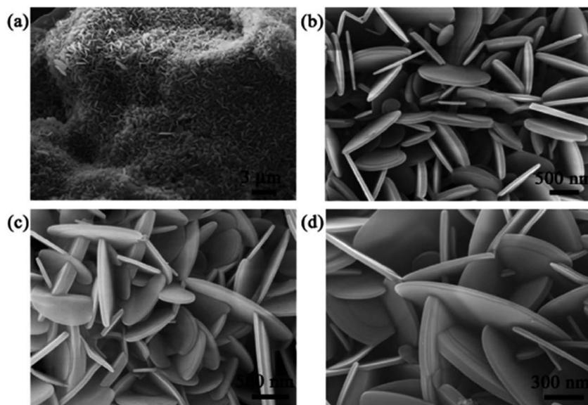
Fig. 11 (a) FE-SEM image and high-resolution FE-SEM images at (b and c) 500 nm and (d) 300 nm of BN nanosheets synthesized at 1200 °C.<sup>80</sup>
