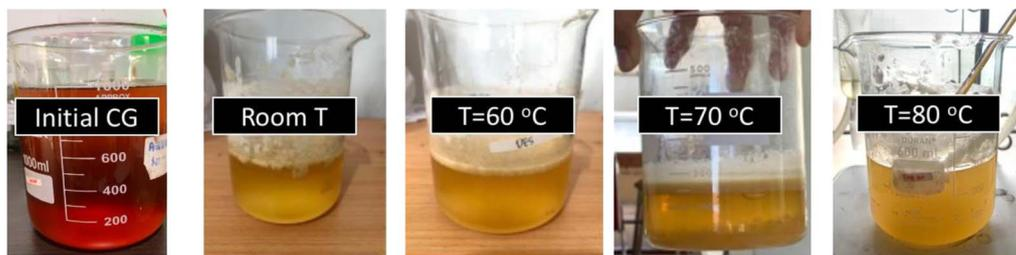
Fig. 4 Crude glycerol after the acidification process with  $\text{H}_3\text{PO}_4$ .
