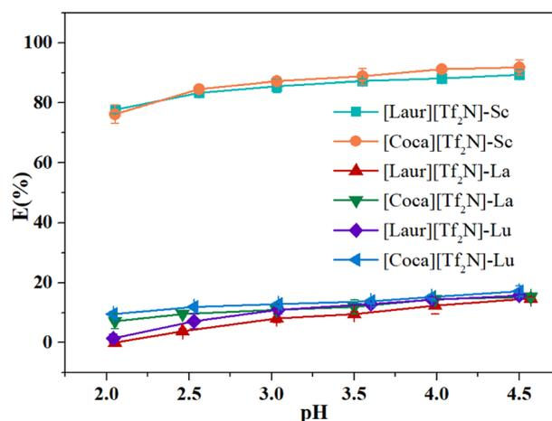
Fig. 10 Extraction efficiency (*E*%) of metal ions by ILs at different pH values of the aqueous phase. Aqueous phase: *V*<sub>aq</sub> = 5 mL, equilibration time = 40 min, *c*<sub>Sc</sub> = *c*<sub>La</sub> = *c*<sub>Lu</sub> = 0.005 mol L<sup>-1</sup>, *c*<sub>NaNO<sub>3</sub></sub> = 0.5 mol L<sup>-1</sup>, and pH = 3. Organic phase: *m*<sub>[Laur][Tf<sub>2</sub>N]</sub> = 0.0816 g and *m*<sub>[Coca][Tf<sub>2</sub>N]</sub> = 0.0921 g.
