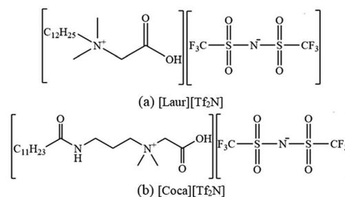
Fig. 1 Structures of the ILs: (a) [Laur][Tf<sub>2</sub>N] and (b) [Coca][Tf<sub>2</sub>N].
