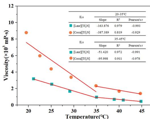
Fig. 3 Viscosity changes and correlation of water-saturated [Laur][Tf<sub>2</sub>N] and [Coca][Tf<sub>2</sub>N] with the increase in temperature.
