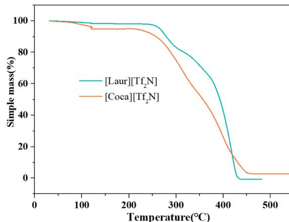
Fig. 2 TGA curves of water-saturated [Laur][Tf<sub>2</sub>N] and [Coca][Tf<sub>2</sub>N].
