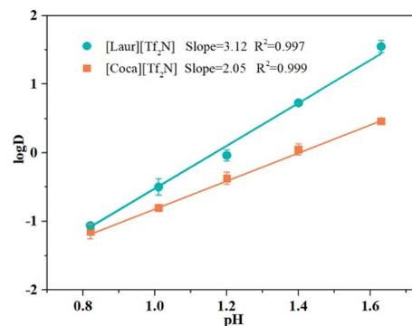
Fig. 5 Plot of logD as a function of pH. Aqueous phase:  $V_{aq} = 5$  mL, equilibration time = 40 min,  $c_{Sc} = 0.0008$  mol L<sup>-1</sup>,  $c_{NaNO_3} = 0.5$  mol L<sup>-1</sup>, and pH = 0.82–1.63. Organic phase:  $V_o = 5$  mL,  $m_{[Laur][Tf_2N]} = 0.1996$  g, and  $m_{[Coca][Tf_2N]} = 0.1768$  g.
