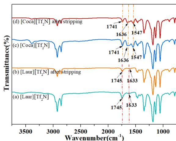
Fig. 8 IR spectra of ILs and ILs after stripping with HNO<sub>3</sub>.
