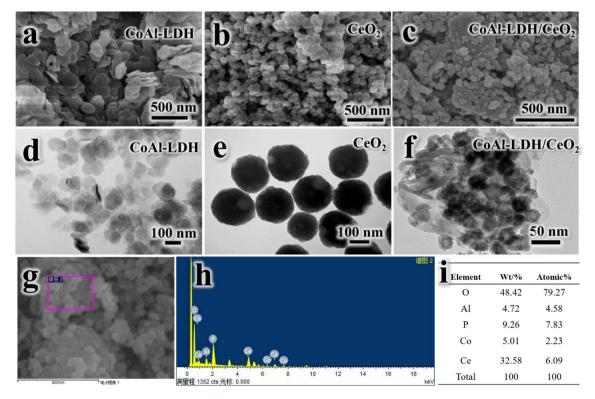
Fig. 2 SEM micrograph for CoAl-LDH (a), CeO<sub>2</sub> (b) and CoAl-LDH/CeO<sub>2</sub> (c), TEM micrograph for CoAl-LDH (d), CeO<sub>2</sub> (e) and CoAl-LDH/CeO<sub>2</sub> (f), element composition and SEM-EDX analysis spectrums of CoAl-LDH/CeO<sub>2</sub> (q-i).
