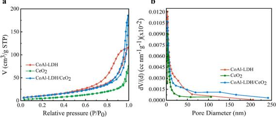
Fig. 5 (a and b) Nitrogen adsorption/desorption isotherms of CoAl-LDH, CeO<sub>2</sub> and CoAl-LDH/CeO<sub>2</sub>.
