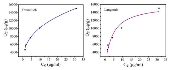
Fig. 6 Adsorption isothermal model of phosphate by CoAl-LDH/CeO<sub>2</sub>
