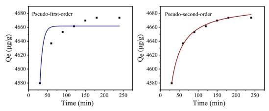
Fig. 7 Adsorption kinetics model of phosphate by CoAl-LDH/CeO<sub>2</sub>.
