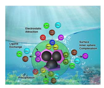
Scheme 1 A schematic diagram of the adsorption mechanism by CoAl-LDH/CeO2.
