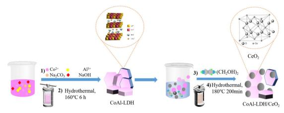
Fig. 1 Schematic process for the facile preparation of CoAl-LDH/CeO<sub>2</sub>.
