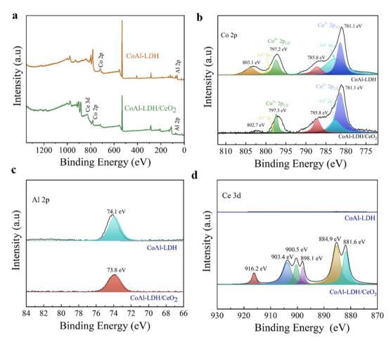
Fig. 4 (a) XPS full spectrum of CoAl-LDH and CoAl-LDH/CeO<sub>2</sub>. High resolution spectra of (b) Co 2p, (c) Al 2p, and (d) Ce 3d of CoAl-LDH and CoAl-LDH/CeO<sub>2</sub>, respectively.
