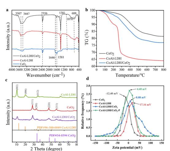
Fig. 3 (a) FT-IR spectra of CoAl-LDH, CeO<sub>2</sub> and CoAl-LDH/CeO<sub>2</sub>. (b) TG curves of CoAl-LDH, CeO<sub>2</sub> and CoAl-LDH/CeO<sub>2</sub>. (c) XRD patterns of CoAl-LDH, CeO2 and CoAl-LDH/CeO2. (d) Zeta potential of the CoAl-LDH, CeO2, CoAl-LDH/CeO2 before and after phosphate adsorption curves
