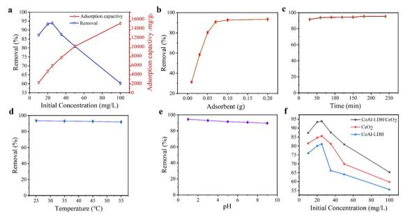
Fig. 8 (a) Effect of initial concentration on removal rate of CoAl-LDH/CeO<sub>2</sub>, (b) effect of CoAl-LDH/CeO<sub>2</sub> dosage on adsorption properties, (c– e) effect of time, temperature and initial solution pH on adsorption properties, respectively, (f) comparison of the adsorption effect of CoAl-LDH, CeO<sub>2</sub> and CoAl-LDH/CeO<sub>2</sub> on phosphate.
