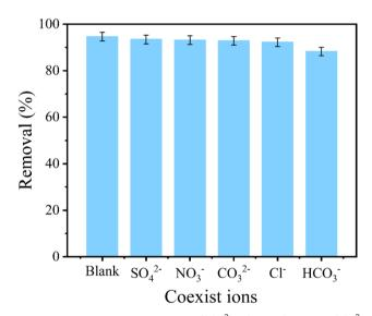
Fig. 9 Effect of coexisting anions ( $SO_4^{2-}$ ,  $Cl^-$ ,  $NO_3^-$  and  $CO_3^{2-}$ ,  $HCO_3^-$ ) on the adsorption of phosphate by CoAl-LDH/CeO<sub>2</sub>.
