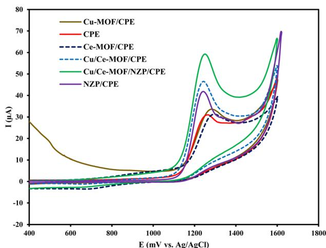
**Fig. 2** Cyclic voltammograms of  $50 \mu\text{mol L}^{-1}$  of target analyte in  $0.10 \text{ mol L}^{-1}$  phosphate buffer solution at the bare CPE, NZP/CPE, Ce-MOF/CPE, Cu-MOF/CPE, Cu/Ce-MOF/CPE and Cu/Ce-MOF/NZP/CPE.
