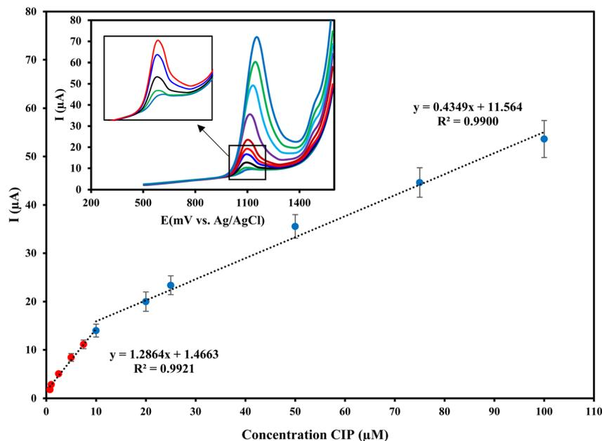
Fig. 7 The calibration curve and linear range of Cu/Ce-MOF/NZP/CPE for determining CIP in 0.1 mol L<sup>-1</sup> phosphate buffer (pH = 3) under optimal conditions (scan rate: 100 mV s<sup>-1</sup>, pulse amplitude: 100 mV). Inset shows the differential pulse voltammograms of CIP.
