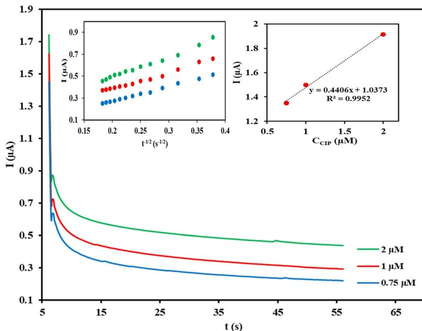
Fig. 4 Chronoamperometry of CIP in 0.1 mol L<sup>-1</sup> phosphate buffer (pH = 3) at three different concentrations (0.75, 1.0, 2.0 μmol L<sup>-1</sup>) with a potential step at 1.1 V at Cu/Ce-MOF/NZP/CPE. Insets show the plot of  $I$  (μA) vs.  $t^{1/2}$  (s<sup>1/2</sup>) obtained from chronoamperograms, and plot of slopes of the linear lines versus CIP concentrations.
