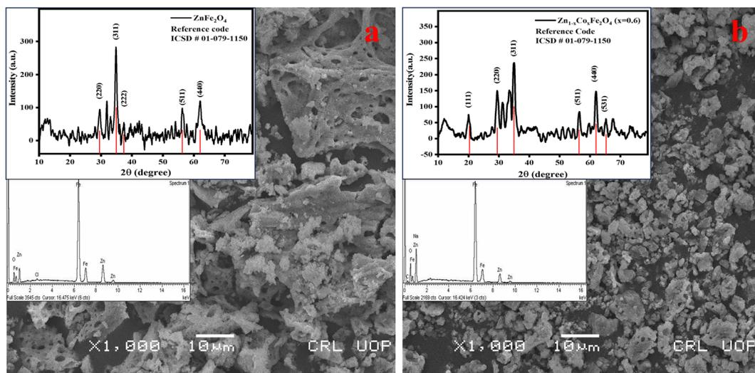
Fig. 2 Scanning electron micrographs along with X-ray diffraction patterns and energy dispersive X-ray spectra for (a)  $\text{ZnFe}_2\text{O}_4$  and (b)  $\text{Zn}_{0.4}\text{Co}_{0.6}\text{Fe}_2\text{O}_4$ .
