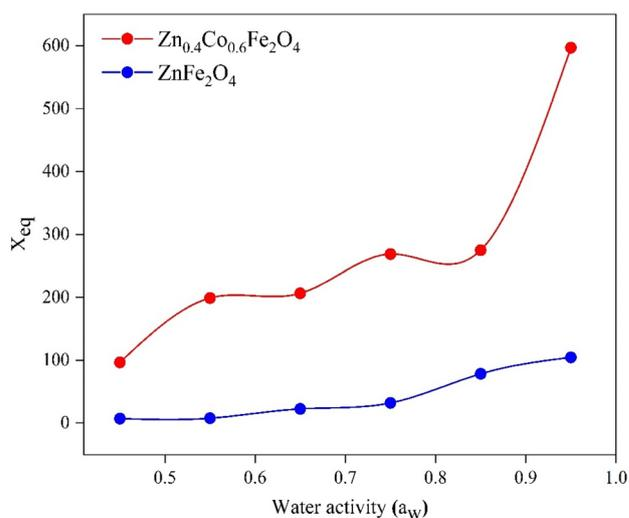
**Fig. 5** Equilibrium moisture content ( $X_{\text{eq}}$ ) versus water activity ( $a_w$ ) for  $\text{ZnFe}_2\text{O}_4$  and  $\text{Zn}_{0.4}\text{Co}_{0.6}\text{Fe}_2\text{O}_4$ .
