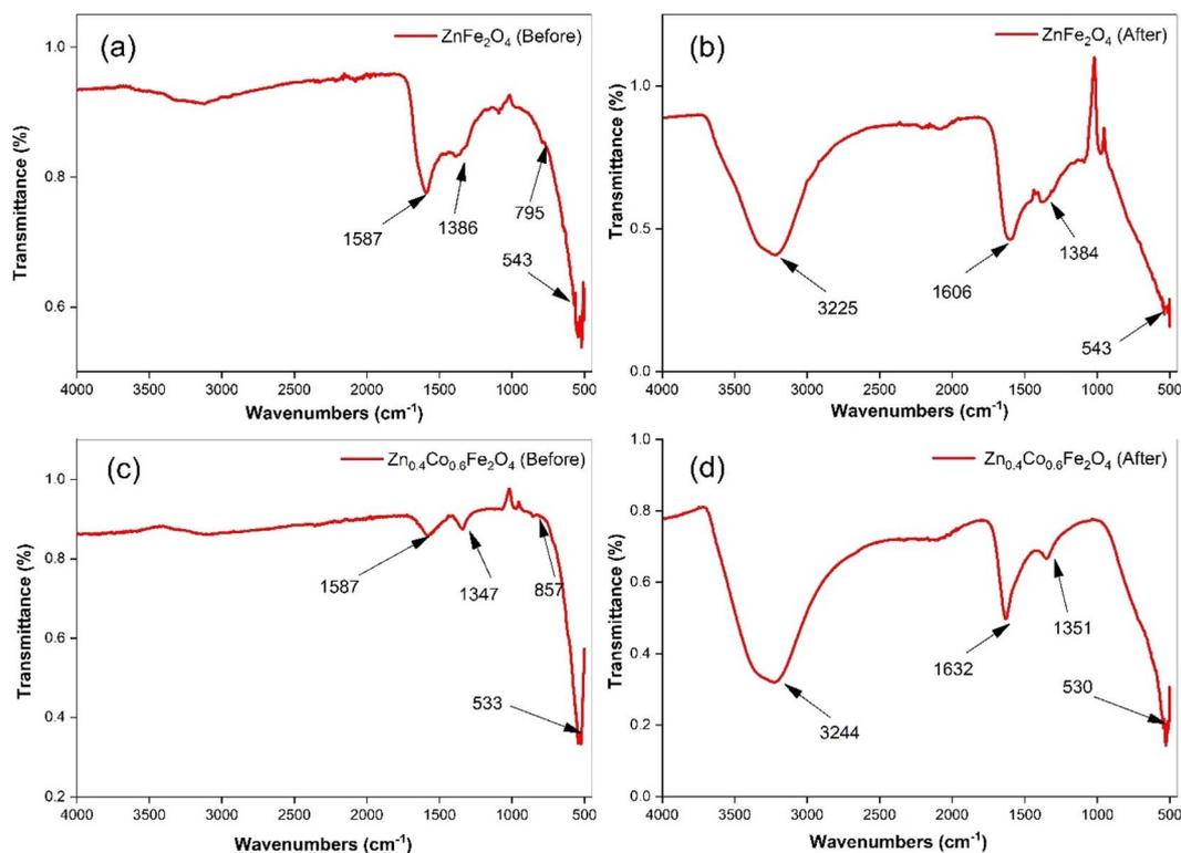
Fig. 3 Fourier-transform infrared spectroscopy for  $\text{ZnFe}_2\text{O}_4$  ((a) before and (b) after adsorption) and  $\text{Zn}_{0.4}\text{Co}_{0.6}\text{Fe}_2\text{O}_4$  ((c) before & (d) after adsorption).
