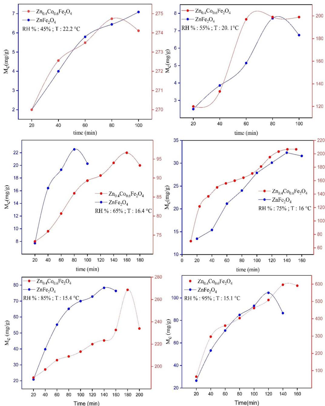
Fig. 4 Graphs of moisture content ( $M_c$ ) versus time for synthesized  $ZnFe_2O_4$  and  $Zn_{0.4}Co_{0.6}Fe_2O_4$  at different RH percentages.
