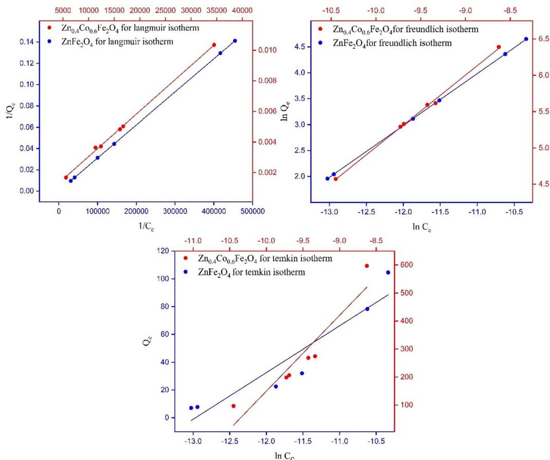
Fig. 6 Fitting of experimental data to various isotherm models for  $\text{ZnFe}_2\text{O}_4$  and  $\text{Zn}_{0.4}\text{Co}_{0.6}\text{Fe}_2\text{O}_4$ .
