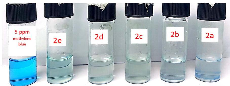
**Fig. 8** Ability of macrocycles **2a–e** to remove methylene blue dye.
