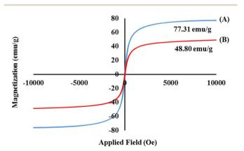
Fig. 3 Hysteresis loop curves of the bare  ${\rm Fe_3O_4}$  MNPs (A) and magnetic cross-linked Pec–Cel hydrogel nanobiocomposite (B).
