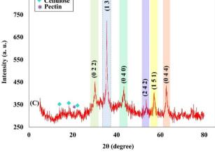
Fig. 1 FTIR spectra of the cross-linked Pec-Cel hydrogel (A) and the magnetic cross-linked Pec-Cel hydrogel nanobiocomposite (B); XRD pattern of the magnetic cross-linked Pec-Cel hydrogel nanobiocomposite structure (C).
