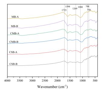
Fig. 2 FTIR spectra of biochar (B-before; A-after).
