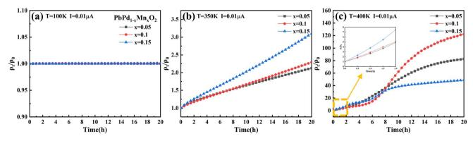
Fig. 5 Time dependence of  $\rho_t/\rho_0$  ratio at (a) T=100 K, (b) T=350 K and (c) T=400 K under the applied constant current of 0.01  $\mu$ A.
