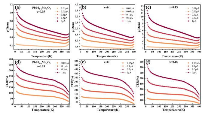
Fig. 2 Temperature dependence of the resistivity of PbPd<sub>1-x</sub>Mn<sub>x</sub>O<sub>2</sub> (x = 0.05, 0.1, 0.15) thin films at different applied currents, (a) x = 0.05, (b) x = 0.05, (b)0.1, (c) x = 0.15. Temperature dependence of CER value of PbPd<sub>1-x</sub>Mn<sub>x</sub>O<sub>2</sub> (x = 0.05, 0.1, 0.15) films, (d) x = 0.05, (e) x = 0.1, (f) x = 0.15.
