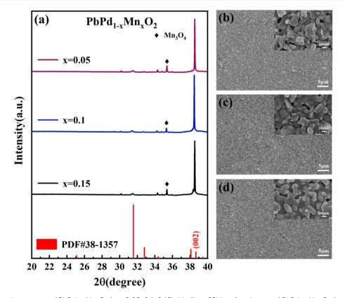
Fig. 1 (a) X-ray diffraction pattern of PbPd<sub>1-x</sub>Mn<sub>x</sub>O<sub>2</sub> (x = 0.05, 0.1, 0.15) thin films SEM surface image of PbPd<sub>1-x</sub>Mn<sub>x</sub>O<sub>2</sub> (x = 0.05, 0.1, 0.15) film, (b) x = 0.05, (c) x = 0.1, (d) x = 0.15.
