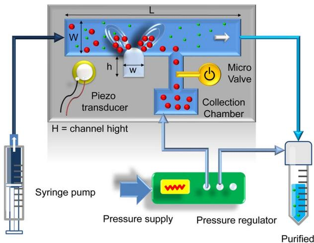
**Fig. 1** Illustration of a microfluidic setup with precise control over flow rate and pressure. This system ensures stable conditions by carefully regulating flow parameters through a syringe pump and a pressure controller. It facilitates continuous and automated size-selective particle removal, allowing captured particles to be directed to a waste outlet or a designated collection chamber.
