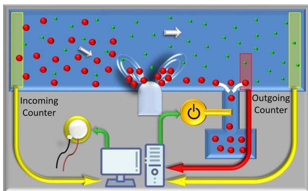
**Fig. 3** Automated particle collection principle: our custom LabVIEW control system manages various functions, including particle counting, piezo transducer and microvalve control, pressure regulation, and flow management. The yellow regions of interest (ROIs) are responsible for particle counting, while the red ROI serves as a sensor to detect particle leaks and trigger valve activation.
