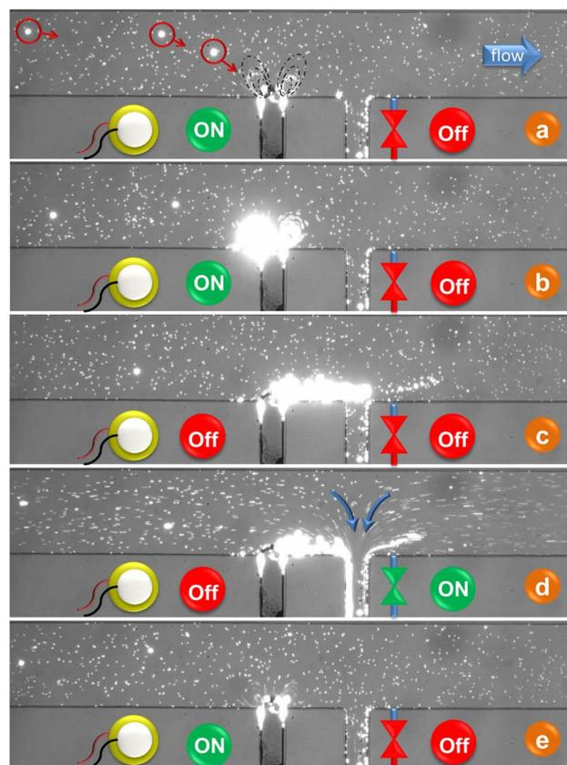
**Fig. 4** Sequential visualization of size-selective particle removal in the microchannel: (a) entrapment of 10 micrometer particles by counter-rotating vortices, (b) augmentation of larger particle concentration, (c) deactivation of the piezo transducer positions larger particles near the exit channel, (d) controlled microvalve opening initiates swift particle suction, (e) repetition of these steps for continuous operation.
