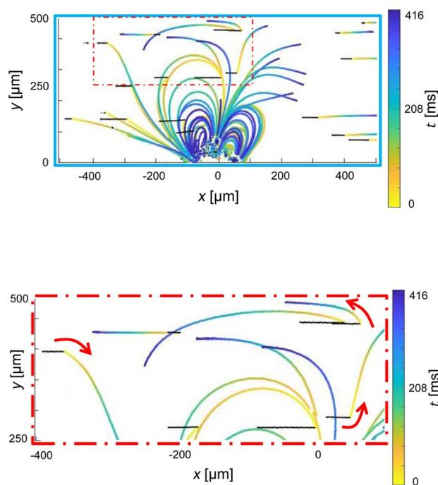
Fig. 6 High-Frequency Micro-Particle Tracking Velocimetry ( $\mu\text{PTV}$ ) at 24 000 frames per second: tracking 2-micrometer particles in the presence of Poiseuille flow (left to right) and microbubble streaming. (a) Presents the entire experimental field of view, while (b) provides an enlarged view (indicated by the red dashed line rectangle) to enhance the visibility of finer details.
