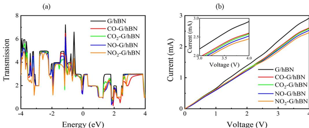
Fig. 8 Transmission spectra at zero bias voltage (a) and current–voltage profile (b) of graphene/h-BN heterostructures upon the adsorption of toxic gases.
