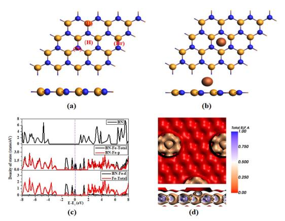
Fig. 1 Optimized geometry of (a) pure (b) Fe-decorated (c) DOS of pure and Fe-decorated h-BN (d) ELF map of Fe decorated h-BN.
