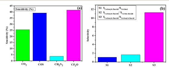
Fig. 4 (a) Sensitivity of the gas sensor based on Fe-decorated h-BN towards gas molecules, including carbon dioxide, carbonyl sulfide, carbimide, and carbonyl fluoride. (b) The selectivity of Fe-decorated h-BN sensor for carbonyl fluoride detection.
