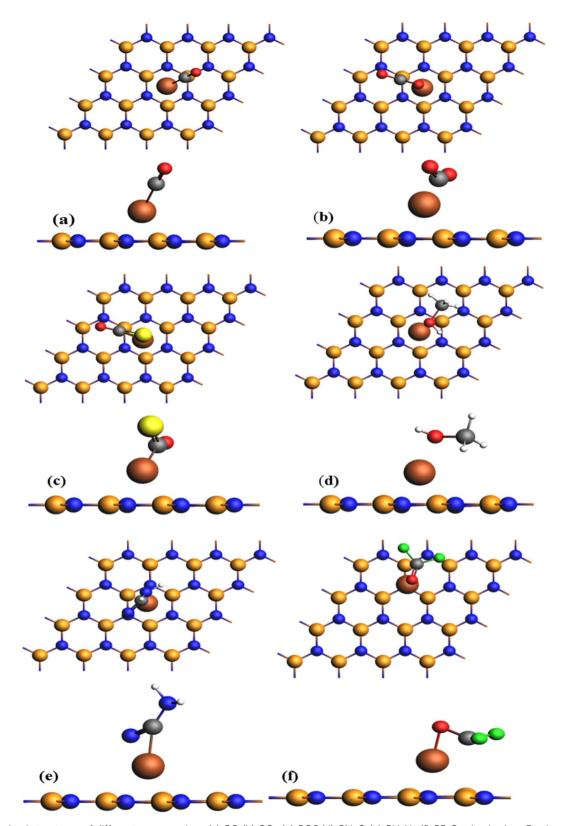
$\textbf{Fig. 2} \quad \textbf{Optimized structures of different gases such as (a) CO (b) CO_2 (c) COS (d) CH_4O (e) CH_2N_2 (f) CF_2O \ adsorbed on Fe-decorated h-BN. } \\$
