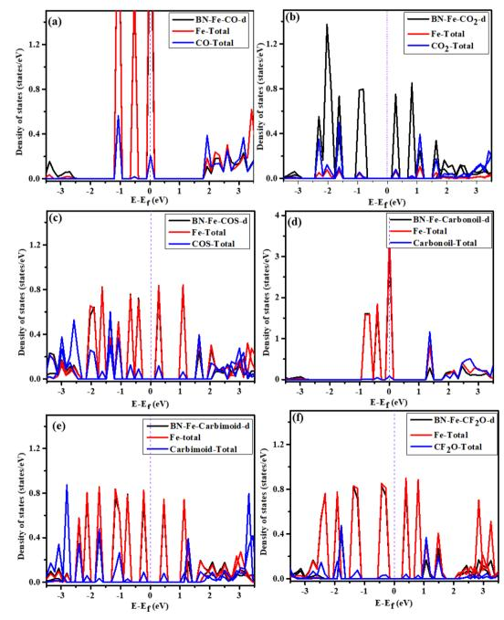
Density of States of the adsorption of (a) CO (b) CO<sub>2</sub> (c) COS (d) CH<sub>4</sub>O (e) CH<sub>2</sub>N<sub>2</sub> (f) CF<sub>2</sub>O gases on Fe-decorated h-BN.
