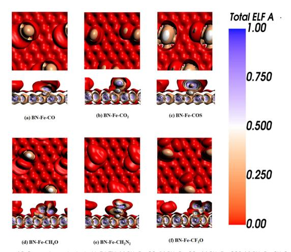
Fig. 5 ELF map of  $B_4C_3$  monolayer adsorbed with 3d-TM. (a) BN-Fe-CO, (b)  $BN-Fe-CO_2$ , (c)  $BN-Fe-CO_3$ , (d)  $BN-Fe-CH_4O$ , (e)  $BN-Fe-CH_2N_2$ , (f)  $BN-Fe-CF_2O$ . The ELF values for the red, white, and blue colored sections are 0.00, 0.50, and 1.0, respectively.
