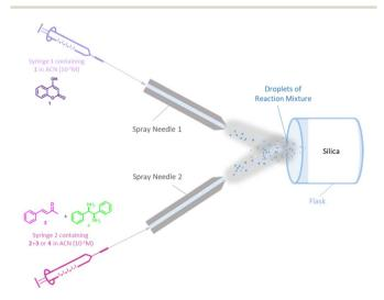
Fig. 2 Simplified scheme of system E. The two spray needles are located at an angle of  $60^{\circ}$ , at the distance of 1 cm from the silica cap.
