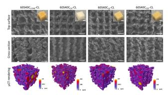
Fig. 4 SEM micrographs and photographs (insets) of 3D printed SiO<sub>2</sub>-CaO/PTHF/PCL-diCOOH hybrids with molar ratio of TEOS: Ca of 60: 40,  $60S40C_{Ca}$ -CL, where Ca is the calcium source used;  $\mu$ CT imaging and analysis of a volume of interest (2600  $\times$  2600  $\times$  2600  $\mu$ m) showing the 3D rendering of the scaffold strut structure, coloured by their diameter size in um.
