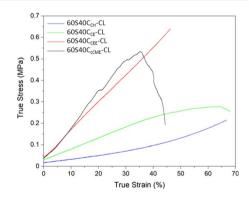
Fig. 5 Typical stress-strain curves of the 3D printed SiO<sub>2</sub>-CaO/PTHF/ PCL-diCOOH hybrids scaffolds with molar ratio of TEOS: Ca of 60: 40, 60S40C<sub>Ca</sub>-CL, where Ca is the calcium source used.
