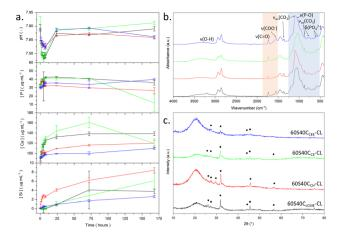
Fig. 3 SBF studies of  $SiO_2$ –CaO/PTHF/PCL-diCOOH hybrid monoliths with molar ratio of TEOS: Ca of 60: 40,  $60S40C_{Ca}$ –CL, where Ca is the calcium source used, post 7 days immersion: (a) pH, phosphorous, calcium, and silicon, concentration measured via ICP-OES. (b) FTIR spectra after immersion; blue region highlights where the bands for calcium phosphate formation are, and the orange region shows bands for the interaction of calcium with the PCL-diCOOH. (c) XRD patterns with HCA peaks.
