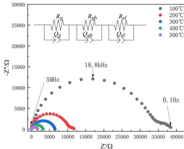
Fig. 5 Partial impedance spectra of SmNiO<sub>3</sub> in 5%H<sub>2</sub>-Ar.
