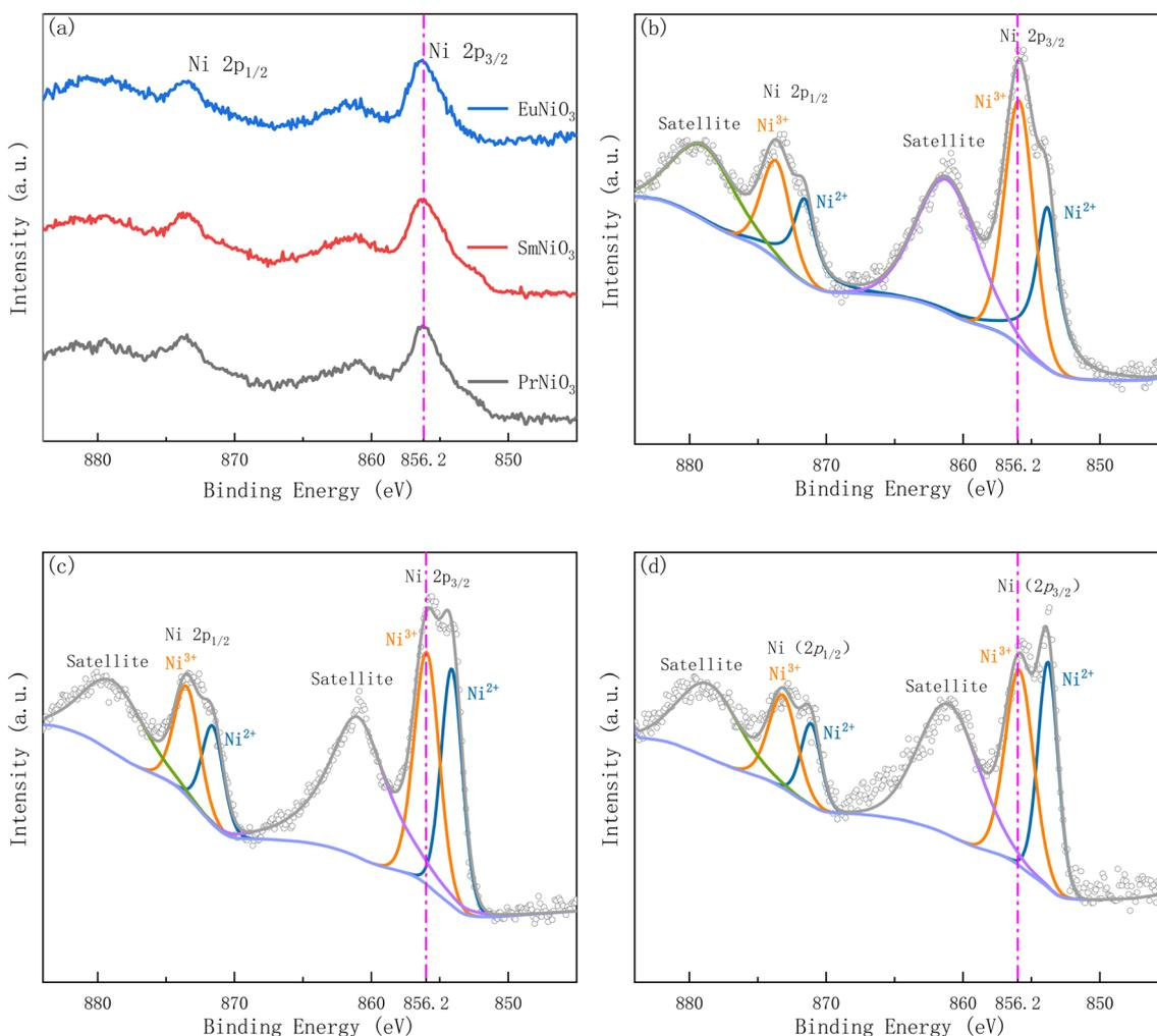
Fig. 3 XPS spectra of three samples before and after 10% $\text{H}_2$ -Ar treatment (a)  $\text{ReNiO}_3$  (Re = Pr, Sm, Eu) before hydrogen treatment (b)  $\text{PrNiO}_3$  after hydrogen treatment (c)  $\text{SmNiO}_3$  after hydrogen treatment (d)  $\text{EuNiO}_3$  after hydrogen treatment.
