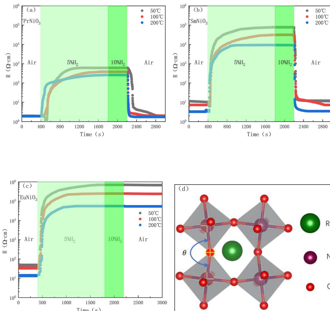
Fig. 2 DC resistivities of three materials in different atmospheres and schematic diagram of crystal structure (a)  $\text{PrNiO}_3$  (b)  $\text{SmNiO}_3$  (c)  $\text{EuNiO}_3$  (d) schematic diagram of  $\text{ReNiO}_3$  crystal structure.
