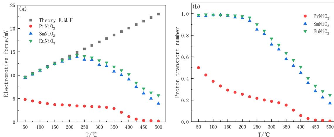
Fig. 4 The EMF (a) and proton transport number (b) of the ReNiO<sub>3</sub>.
