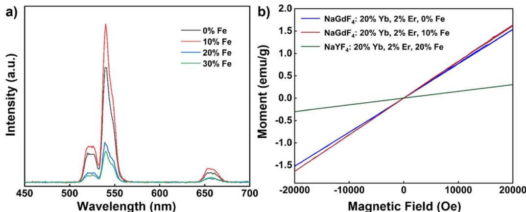
Fig. 7 (a) Upconversion emission spectra of NaGdF<sub>4</sub>: 20% Yb, 2% Er, x% Fe (x = 0, 10, 20, 30) nanoparticles (980 nm continuous excitation, excitation power density: 2 W cm<sup>-2</sup>). (b) Magnetic susceptibility of NaGdF<sub>4</sub>: 20% Yb, 2% Er, 0% Fe, NaGdF<sub>4</sub>: 20% Yb, 2% Er, 10% Fe and NaYF<sub>4</sub>: 20% Yb, 2% Er, 20% Fe nanocrystals.
