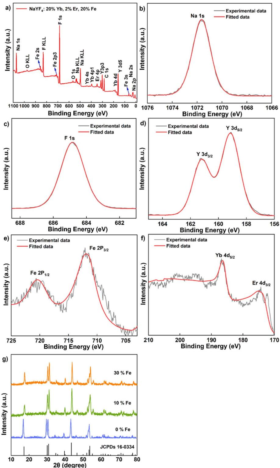
Fig. 2 (a–f) XPS spectrum of the sample NaYF<sub>4</sub>: 20% Yb, 2% Er, 20% Fe. (g) XRD data of the samples NaYF<sub>4</sub>: 20% Yb, 2% Er, x% Fe (x = 0, 10, 30).
