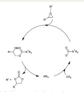
Fig. 2 Possible mechanism of cyclic carbonate formation including  ${\rm CO_2}$  activation by tertiary amine.
