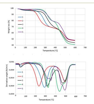
Fig. 4 Thermogravimetric curves recorded for 1–5 under the nitrogen atmosphere.
