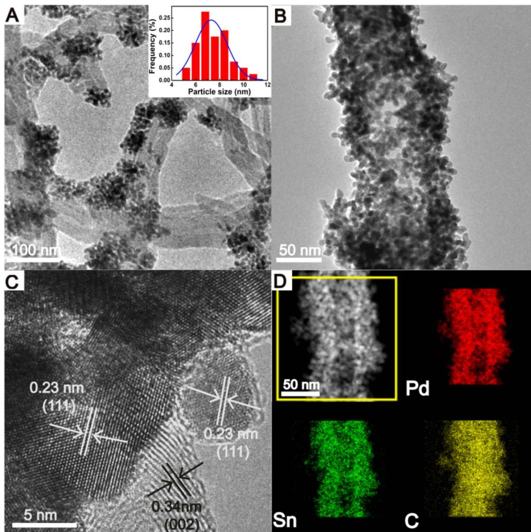
Fig. 3 (A and B) The low- (A) and high- (B) magnification TEM images of the typical Pd<sub>3</sub>Sn/CNTs NHs. (C) HRTEM image for the Pd<sub>3</sub>Sn NCs on an individual CNT. (D) Corresponding HAADF-STEM image and elemental mapping for Pd<sub>3</sub>Sn/CNT NHs.
