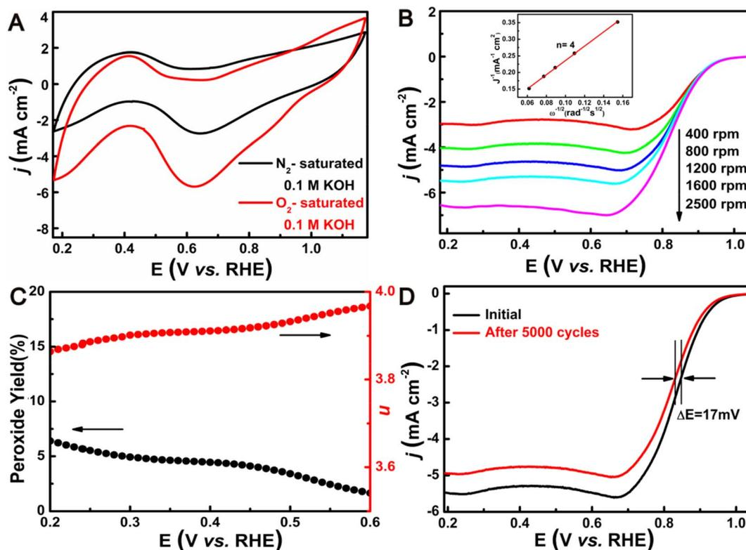
Fig. 4 (A) The CVs of Pd<sub>3</sub>Sn/CNTs NHs. (B) ORR polarization plots of Pd<sub>3</sub>Sn/CNTs NHs at different rotating rates. (C) The peroxide species yield (black color) and the number of transferred electrons (*n*) (red color) of Pd<sub>3</sub>Sn/CNTs NHs. (D) The durability test for Pd<sub>3</sub>Sn/CNTs NHs.
