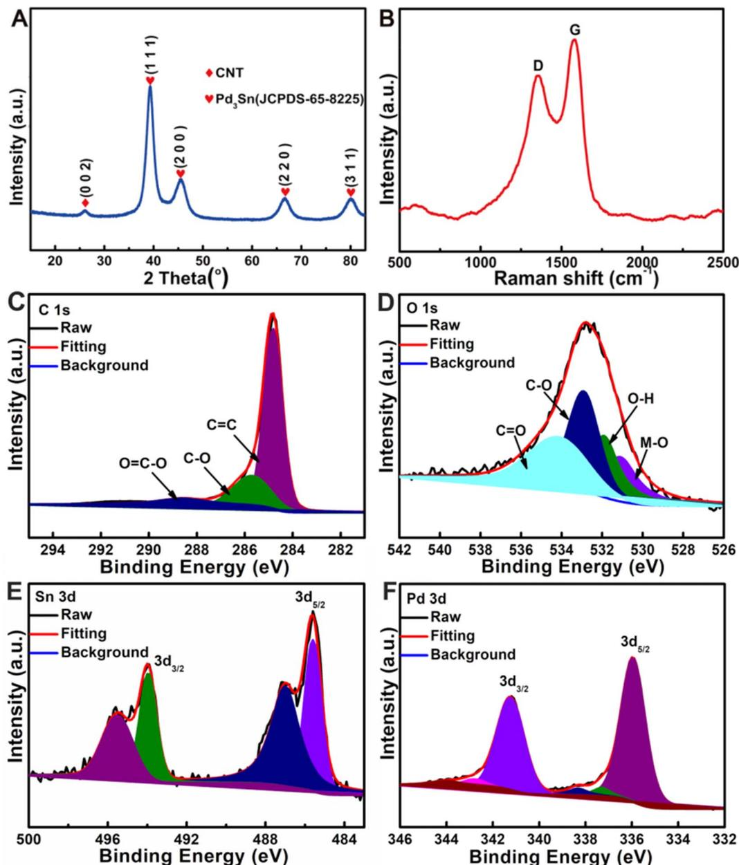
Fig. 2 (A and B) XRD pattern (A) and Raman spectra (B) of Pd<sub>3</sub>Sn/CNT NHs. (C–F) The C 1s (C), O 1s (D), Sn 3d (E), and Pd 3d (F) fine XPS spectra for the typical Pd<sub>3</sub>Sn/CNT NHs.
