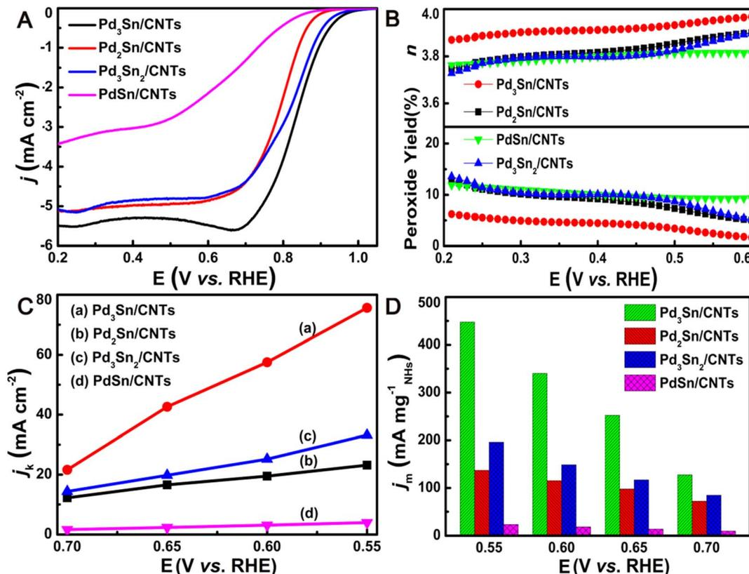
Fig. 5 (A) ORR polarization plots of the  $\text{Pd}_x\text{Sn}_y/\text{CNTs}$  NHs at 1600 rpm. (B) The peroxide species yield and the number of transferred electrons ( $n$ ) of  $\text{Pd}_x\text{Sn}_y/\text{CNTs}$  NHs. (C) Kinetic current density ( $j_k$ ) versus potential plots for those  $\text{Pd}_x\text{Sn}_y/\text{CNTs}$  NHs. (D) Mass-specific activities of  $\text{Pd}_x\text{Sn}_y/\text{CNTs}$  NHs.
