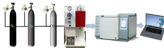
Fig. 2 Adsorption device of Na-X for a low concentration of CO<sub>2</sub>.
