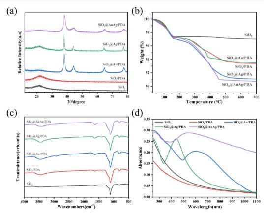
Fig. 4 (a) XRD diffraction patterns, (b) TG curves, (c) FTIR spectra and (d) UV-vis absorption spectra of SiO<sub>2</sub>, SiO<sub>2</sub>/PDA, SiO<sub>2</sub>@Au/PDA, SiO<sub>2</sub>@Ag/PDA and SiO<sub>2</sub>@AuAg/PDA.
