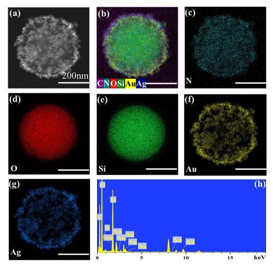
$\textbf{Fig. 2} \quad \text{HAADF-STEM images and EDX elemental mapping of C, N, O, Si, Au and Ag (a-g), and EDX spectrum of SiO_2@AuAg/PDA (h); scale bars are also considered as a scale bar of the scale bars are also considered as a scale bar of the scale bars are also considered as a scale bar of the sca$ 200 nm.
