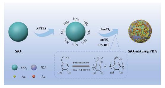
Scheme 1 Schematic illustration for the preparation of SiO<sub>2</sub>@AuAq/PDA core/shell nanospheres.
