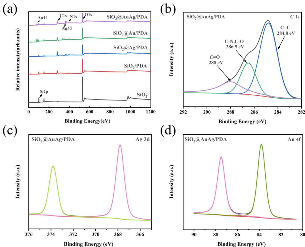
Fig. 5 (a) XPS of  $\text{SiO}_2$ ,  $\text{SiO}_2/\text{PDA}$ ,  $\text{SiO}_2@Ag/\text{PDA}$ ,  $\text{SiO}_2@Au/\text{PDA}$  and  $\text{SiO}_2@AuAg/\text{PDA}$ ; (b) C 1s, (c) Ag 3d and (d) Au 4f core-level spectra of  $\text{SiO}_2@AuAg/\text{PDA}$ .
