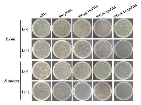
Fig. 8 Images of bacteria colonies formed by E. coli and S. aureus treated with  $SiO_2$ ,  $SiO_2$ /PDA,  $SiO_2$ @Au/PDA,  $SiO_2$ @Ag/PDA and  $SiO_2$ @AuAg/PDA (60  $\mu$ g mL $^{-1}$ ) with or without NIR irradiation for 6 min (808 nm, 2.5 W cm $^{-2}$ ).
