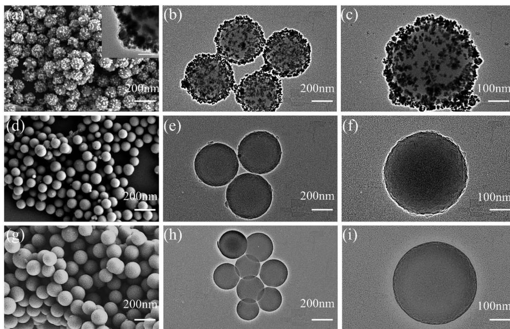
Fig. 1 SEM (a) and TEM (b and c) images of  $\text{SiO}_2\text{@AuAg/PDA}$ , SEM (d) and TEM (e and f) images of  $\text{SiO}_2\text{/PDA}$ , and SEM (g) and TEM (h and i) images of  $\text{SiO}_2$ ; the scale bar of the TEM inset in (a) is 20 nm.
