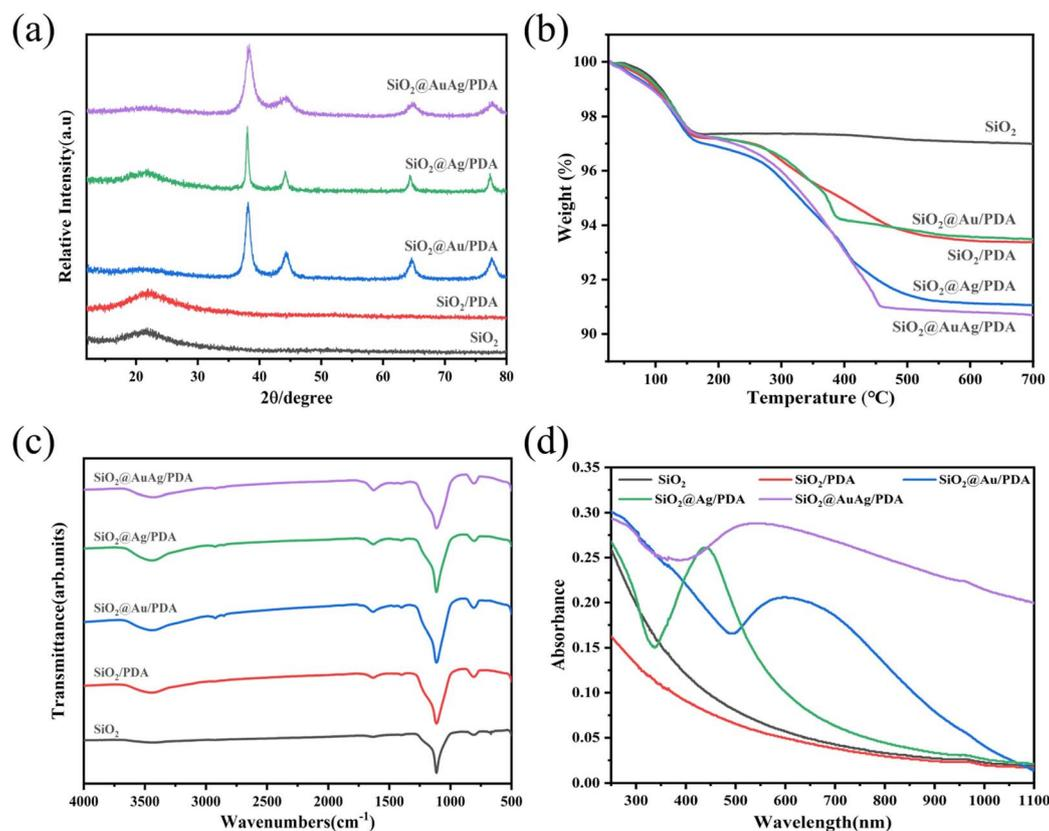
Fig. 4 (a) XRD diffraction patterns, (b) TG curves, (c) FTIR spectra and (d) UV-vis absorption spectra of  $\text{SiO}_2$ ,  $\text{SiO}_2$ /PDA,  $\text{SiO}_2$ @Au/PDA,  $\text{SiO}_2$ @Ag/PDA and  $\text{SiO}_2$ @AuAg/PDA.
