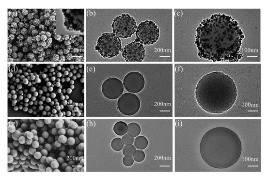
Fig. 1 SEM (a) and TEM (b and c) images of  $SiO_2$ @AuAg/PDA, SEM (d) and TEM (e and f) images of  $SiO_2$ /PDA, and SEM (g) and TEM (h and i) images of  $SiO_2$ ; the scale bar of the TEM inset in (a) is 20 nm.
