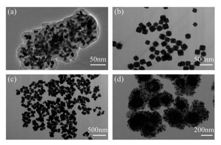
Fig. 3 TEM images of AuAg/PDA (a), ZIF-8 (b), and ZIF-8@AuAg/PDA (c and d).
