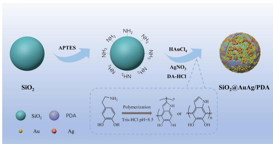
Scheme 1 Schematic illustration for the preparation of SiO<sub>2</sub>@AuAg/PDA core/shell nanospheres.
