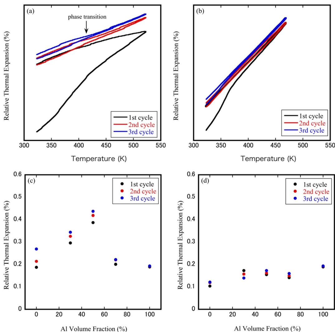
Fig. 4 TMA curves of (a) Al 50 vol%  $ZrW_2O_8/Al$  specimen and (b) Al 50 vol%  $ZrWMoO_8/Al$  specimen subjected to three heating-cooling cycles; change in the CTEs after heating cycle as a function of the volume fraction of (c)  $ZrW_2O_8/Al$  specimens and (d)  $ZrWMoO_8/Al$  specimens for three cycles.
