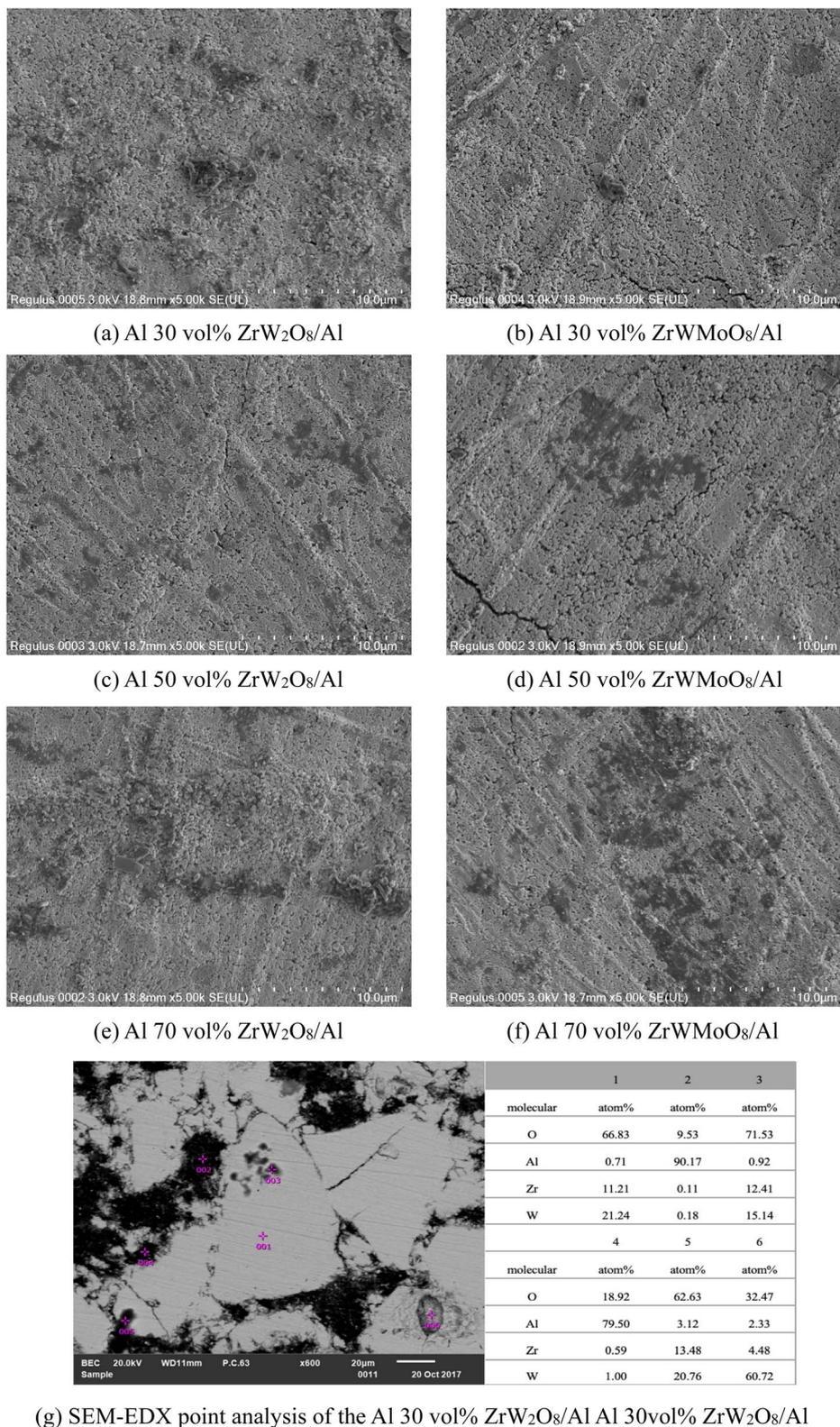
Fig. 3 (a–f) SEM images of the polished surface of ZrW<sub>2-x</sub>Mo<sub>x</sub>O<sub>8</sub>/Al ( $x = 0.0, 1.0$ ) composites; (g) SEM-EDX point analysis of the Al 30 vol% ZrW<sub>2</sub>O<sub>8</sub>/Al specimen.
