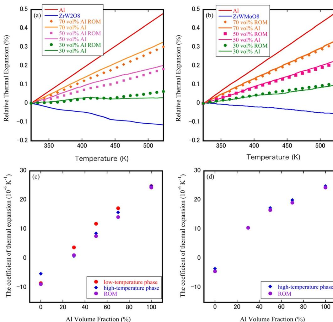
Fig. 5 TMA curves of (a)  $\text{ZrW}_2\text{O}_8/\text{Al}$  and (b)  $\text{ZrWMoO}_8/\text{Al}$  composites during the third heating cycle; CTEs of (c)  $\text{ZrW}_2\text{O}_8/\text{Al}$  and (d)  $\text{ZrWMoO}_8/\text{Al}$  composites.
