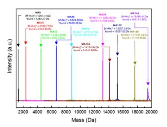
Fig. 2 Combined MALDI-TOF mass spectra of uPMAs.
