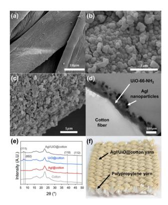
Fig. 1 SEM images of (a) carboxymethylated cotton, (b) UiO@cotton, and (c) Agl/UiO@cotton. (d) TEM image of Agl/UiO@cotton. (e) XRD data of cotton, Agl@cotton, UiO@cotton, and Agl/UiO@cotton. (f) Photograph of floating Agl/UiO@fabric in woven construction.
